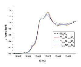
Figure 7. Normalised XANES Nb<sub>2</sub>O<sub>5</sub>, Ti<sub>0.97</sub>Nb<sub>0.03</sub>O<sub>2</sub>, Ti<sub>0.92</sub>Nb<sub>0.08</sub>O<sub>2</sub> and Ti<sub>0.77</sub>Nb<sub>0.23</sub>O<sub>2</sub> thin films.
