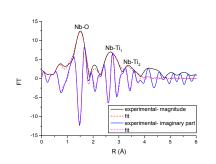
Figure 9. Nb K-edge EXAFS of Ti<sub>0.37</sub>Nb<sub>0.03</sub>O<sub>2</sub> thin film a) plot showing the  $k^{3}\chi(k)$  b) plot showing the magnitude and imaginary part of the Fourier transform of the Nb K-edge EXAFS data of the Ti<sub>0.57</sub>Nb<sub>0.03</sub>O<sub>2</sub> thin film.
