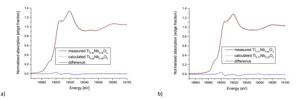
Figure 8. Normalised XANES spectrum along with linear combination of a)  $Ti_{0.92}Nb_{0.08}O_2$  sample containing: 10.8 %  $Nb_2O_5$  and 89.2% as-deposited  $Ti_{0.97}Nb_{0.03}O_2$  sample and b)  $Ti_{0.77}Nb_{0.23}O_2$  sample containing: 48.4% of  $Nb_2O_5$  and 51.6 % of as-deposited  $Ti_{0.97}Nb_{0.03}O_2$  sample.
