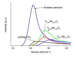
Figure 4. Shift of  $\mathsf{E}_g$  band of niobium doped  $\mathsf{TiO}_2$  and pristine titania films formed from the AACVD compared to anatase powder
