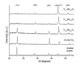
Figure 2. XRD pattern of anatase powder and Nb doped titania films prepared by AACVD at on silica coated glass. The anatase reflection positions with appropriate values (h k l) are shown in brackets.
