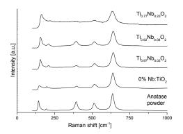
Figure 3. Raman spectra of anatase powder and as-deposited Nb doped titania films on silica coated glass.
