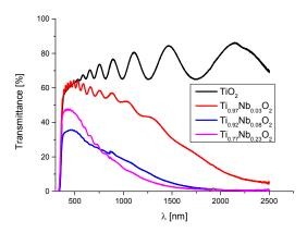
Figure 11. Transmittance (%) plot of as-deposited niobium doped titania thin films over the UV-vis-IR range.
