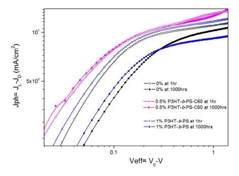
**Figure 13.** Experimental photocurrents after 1 h and 1000 h as a function of  $V_{\rm eff}$  for hero cells of: P3HT:PCBM reference (black curves, circular symbol); P3HT:PCBM and 1wt% P3HT-b-PS (blue curves, triangle symbol); and P3HT:PCBM and 0.5wt% P3HT-b-PS-C<sub>60</sub> (magenta curves, square symbol).
