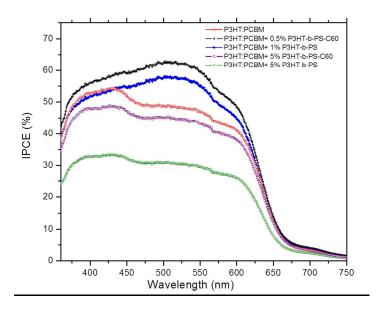
**Figure 10.** IPCE (%) spectra of P3HT: PCBM with varying wt% fractions of added P3HT-b-PS-C<sub>60</sub> (all following annealing at 165 °C, 10 min).
