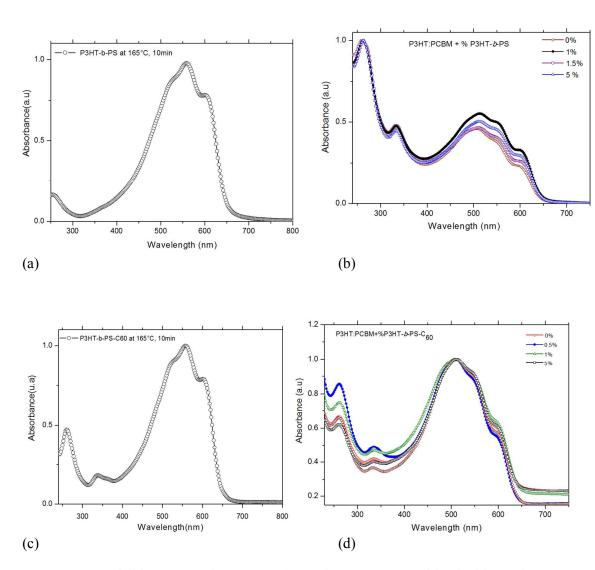
**Figure 3.** UV-visible spectra of: (a) P3HT-*b*-PS; (b) P3HT:PCBM blend with varying wt% loads of P3HT-*b*-PS; (c) P3HT-*b*-PS-C<sub>60</sub>; and (d) P3HT:PCBM with varying wt% loads of P3HT-*b*-PS-*b*-C<sub>60</sub> (all annealed at 165 °C, 10 min).
