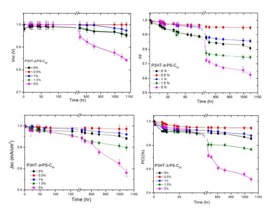
**Figure 12.** Decay curves under illumination of  $V_{oc}$ , FF,  $J_{sc}$  and PCE (%) of P3HT:PCBM based devices with varying wt% fractions of P3HT-b-PS-C<sub>60</sub>. All performed in glove-box under nitrogen.
