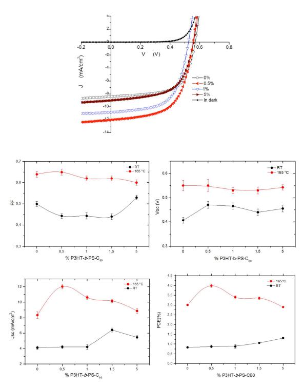
**Figure 9.** Photovoltaic characteristics of P3HT:PCBM blended with various %wt of P3HT-b-PS-b-C<sub>60</sub>: (top) J-V characteristics; (below) FF,  $V_{\rm oc}$ ,  $J_{\rm sc}$ , and PCE (%), obtained with as-cast (black) and annealed (red) solar cells. Error bars were calculated from an average over 16 devices.
