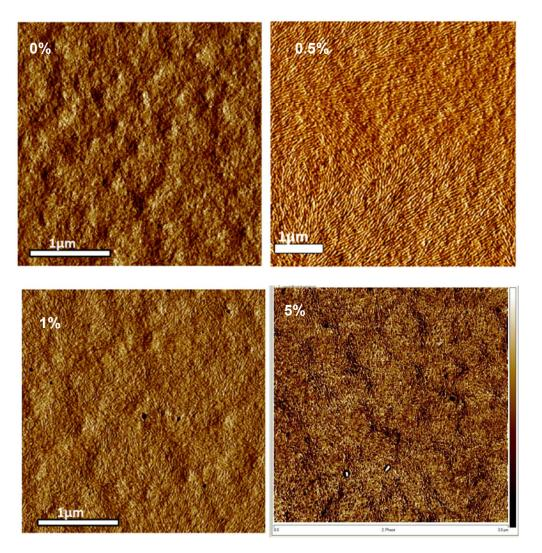
**Figure 6**. AFM images of P3HT:PCBM blends mixed with varying wt% loads of P3HT-b-PS-C<sub>60</sub>, (all 3 × 3  $\mu$ m tapping mode of samples annealed at 165 °C, 10 min).
