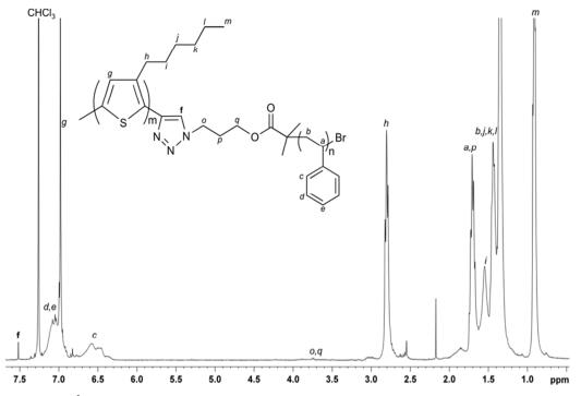
Figure 2. <sup>1</sup>H NMR (400 MHz, CDCl<sub>3</sub>) spectrum of P3HT-*b*-PS.
