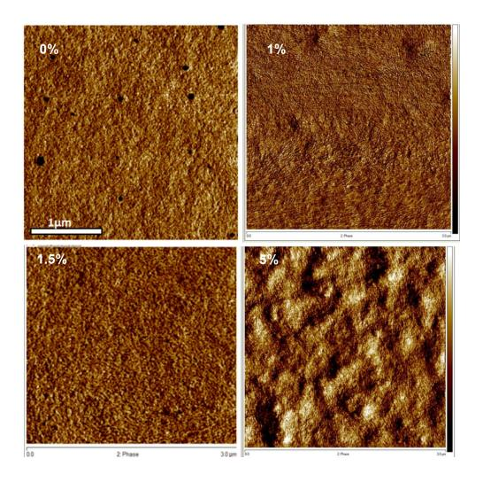
**Figure 4.** AFM phase images of P3HT:PCBM blends mixed with varying wt% loads of P3HT-b-PS, (all 3  $\times$  3  $\mu$ m tapping mode of samples annealed at 165 °C, 10 min).
