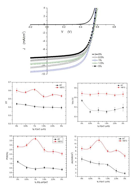
**Figure 8**: Photovoltaic characteristics of P3HT:PCBM blended with various %wt of P3HT-b-PS: (top) J-V characteristics; (below) FF,  $V_{oc}$ ,  $J_{sc}$ , and PCE (%), obtained with as-cast (black) and annealed (red) solar cells. Error bars were calculated from an average over 16 devices.
