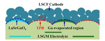
Fig. 24 (a) Schematic diagrams for the interfaces and TPBs between cathode and electrolytes prepared by powder A 27x10mm (300 x 300 DPI)
