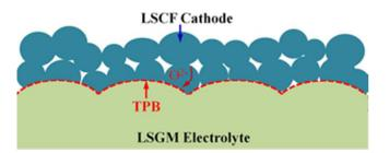
Fig. 24 (b) Schematic diagrams for the interfaces and TPBs between cathode and electrolytes prepared by powder B 27x10mm (300 x 300 DPI)
