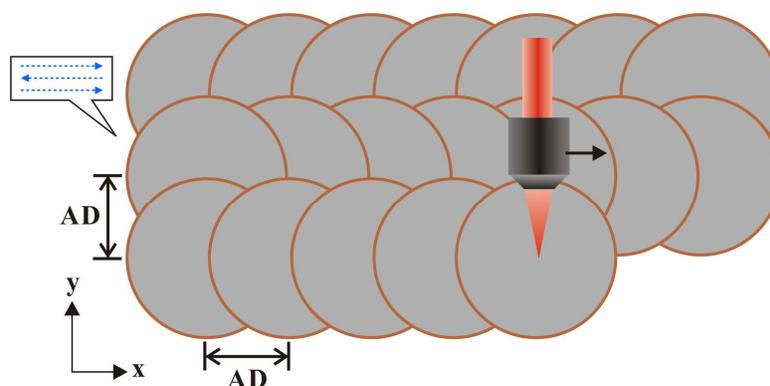
**Figure 2.** Schematic illustration of the scanning process and the detailed definition of *AD*.
