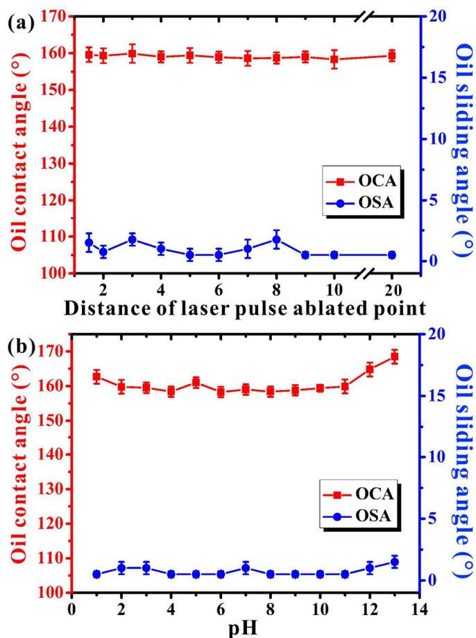
**Figure 6.** (a) Oil contact/sliding angles of underwater oil droplet on the as-prepared surface fabricating at different average distances of laser pulse ablated point. (b) Dependences of the oil contact/sliding angles on the pH of water solution.
