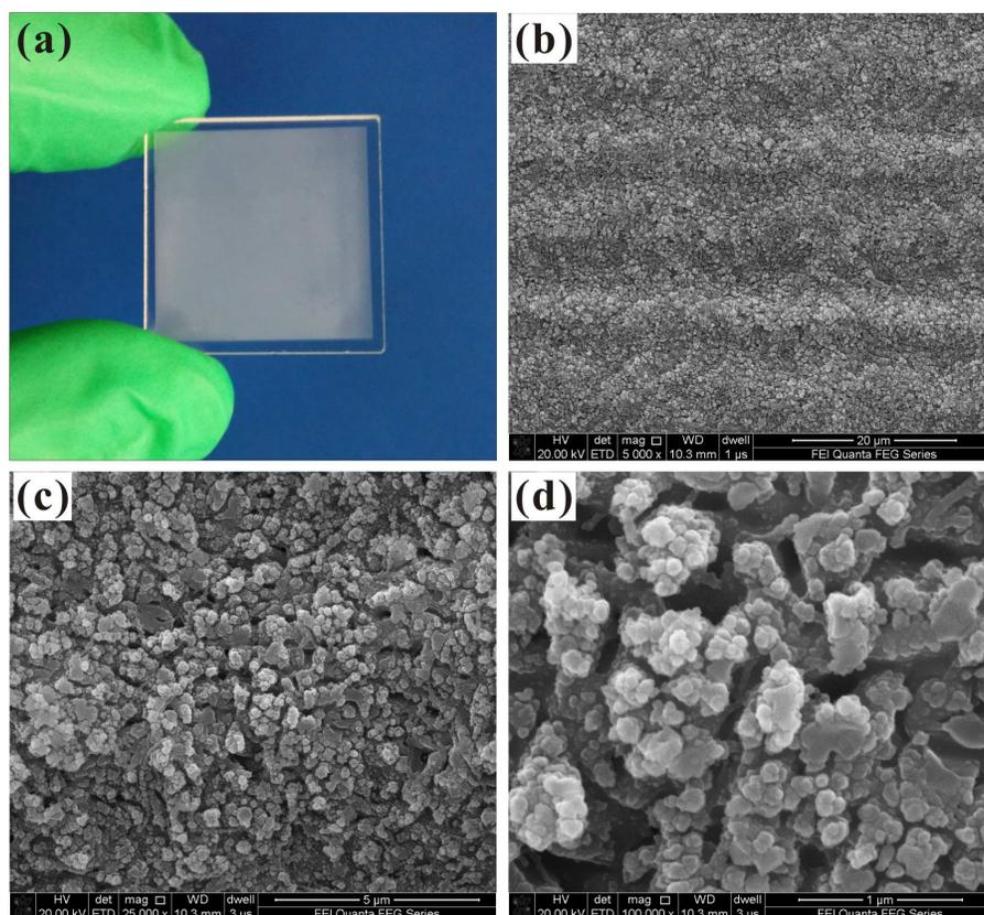
**Figure 3.** (a) Digital image of the femtosecond laser irradiated silica glass with the total size of  $2 \times 2 \text{ cm}^2$ . (b-d) SEM images of laser-induced microstructure with different magnifications.
