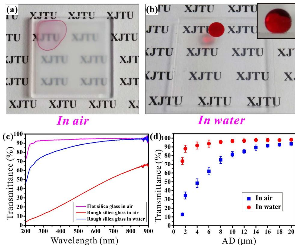
**Figure 5.** (a,b) Images of the as-prepared surface ( $AD = 4 \mu\text{m}$ ) on a piece of paper in different medium: (a) in air; (b) in water. (c) UV-vis spectra of femtosecond laser ablated silica glass ( $AD = 4 \mu\text{m}$ ). (d) Variation of transmittance of the femtosecond laser ablated silica glass with the average distance of laser pulse ablated point.
