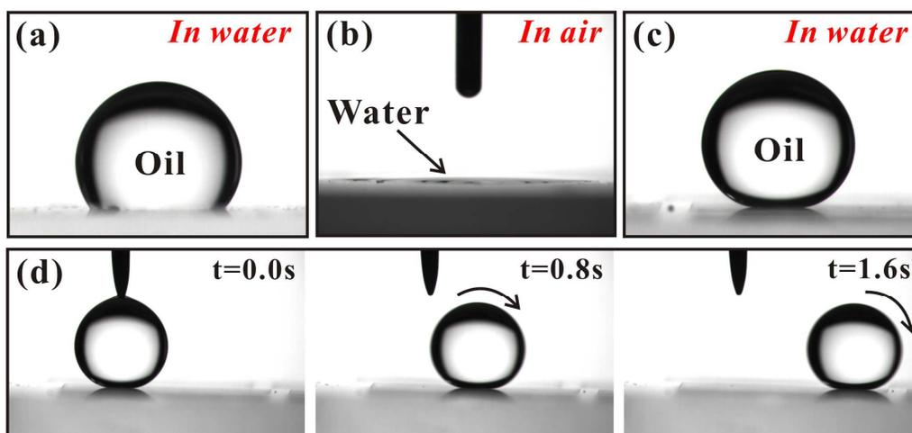
**Figure 4.** Wettability of the femtosecond laser irradiated silica glass ( $AD = 4 \mu\text{m}$ ). (a) An oil droplet on the unstructured silica glass sample in water. (b) A water droplet spreading on the as-prepared rough surface in air medium. (c) Shape of an oil droplet on the laser-induced surface with OCA of  $160.2 \pm 1^\circ$  in water medium. (d) An oil droplet rolling off on a  $1^\circ$  tilted sample.
