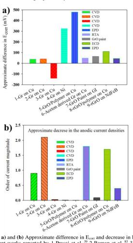
**Fig. 8 a)** and **(b)** Approximate difference in  $E_{corr}$  and decrease in  $I_{corr}$  for different works reported by 1-Prasai et al.,<sup>39</sup> 2-Raman et al.,<sup>83</sup> 3- & 4-Kirkland et al.,<sup>77</sup> 5-Singh et al.,<sup>46</sup> 6-Huh et al.,<sup>44</sup> 7-Krishnamoorthy et al.,<sup>57</sup> 8-Sahu et al.,<sup>80</sup> 9-He et al.<sup>45</sup>
