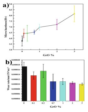
**Fig. 14 (a)** The microhardness of GrO/UHMWPE composites with the different GrO contents; **(b)** Variation of wear rate of the GrO/UHMWPE composites as a function of GrO content after the wear tests.<sup>110</sup> (Reprinted with permission from ref. 14. Copyright (2012) Springer)
