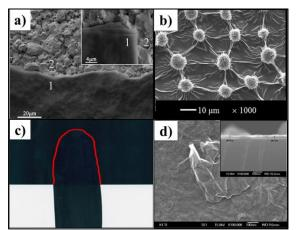
**Fig. 5** Different approaches of Gr based corrosion protective coating; a) Electrophoretic deposition of GrO;<sup>45</sup> b) Templated epoxy/Gr based hydrophobic coating;<sup>60</sup> c) GrO nanopaint;<sup>57</sup> d) Layer-by-layer deposition of GrO and poly(ethylenimine).<sup>61</sup> (Reprinted with permission from ref. 45, 60, 57, and 61. Copyright (2013, 2014, 2014, 2012 respectively) Elsevier.)
