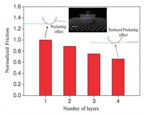
**Fig. 15** Mechanism of reducing puckering effect by multi-layer Gr;<sup>120</sup> (Reprinted with permission from ref. 120. Copyright (2010) AAAS)
