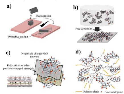
Fig. 2 Film formation mechanism of Gr and GrO, a) Physical deposition and subsequent curing, b) Self-assembly, c) Layer by layer deposition and d) Sol-gel process
