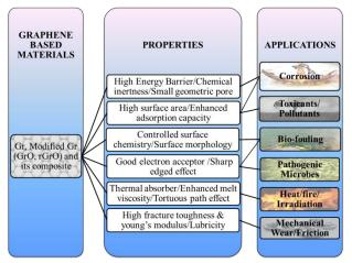
Fig. 1 Protective applications for graphene based materials
