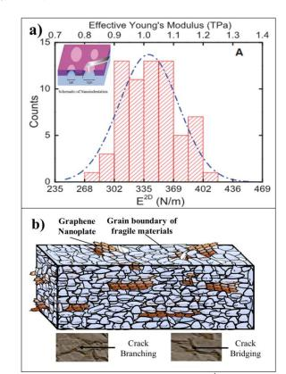
**Fig. 11 (a)** Histogram of elastic stiffness of Gr.<sup>4</sup> (b) Strengthening mechanism of fragile materials by Gr. (Reprinted with permission from ref. 4. Copyright (2008) AAAS)
