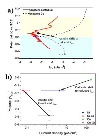
**Fig. 7** Result of potentiodynamic polarization of the Gr and GrO based coating by different coating applicator (NaCl solution); (a) CVD grown Gr on Cu-Positive Shift of  $I_{corr}$  (0.1 M NaCl);<sup>83</sup> (b) CVD grown Gr on Ni-Positive shift of  $I_{corr}$  and Cu- negative shift of  $I_{corr}$ ,<sup>77</sup> (Reprinted with permission from ref. 83 and 77. Copyright (2012, 2012 respectively) Elsevier)
