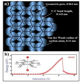
**Fig. 3** (a) Close packed atomic structure of single layer Gr sheet, (b) Energy barriers singlet (nonmagnetic)  $O_2$ , which are forced to pass from the top to the bottom side of Gr.<sup>6</sup> (Reprinted with permission from ref. 6. Copyright (2012) American Physical Society)
