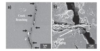
**Fig. 12** (a) Crack branching at platelets with lower dimension characteristic for the systems; b) Crack bridging by platelet with the plane orientated nearly perpendicularly to the plane of the section.<sup>103</sup> (Reprinted with permission from ref. 103. Copyright (2012) Elsevier)
