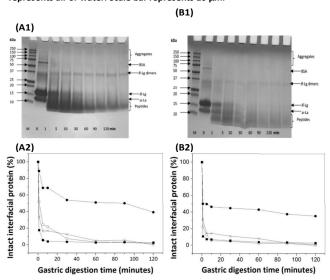
Figure 6. Reduced SDS-PAGE patterns (i) and quantification of intact protein bands (ii) obtained from adsorbed phase of whey protein microgel-stablized emulsions during gastric digestion with added pepsin: A, non-heated; B, heat treated. Symbols represent intact  $\theta$ -Lg monomer (o), $\theta$ -Lg dimer ( $\bullet$ ), BSA ( $\blacksquare$ ) and  $\alpha$ -La ( $\times$ ) at the interface as a function of gastric digestion time.
