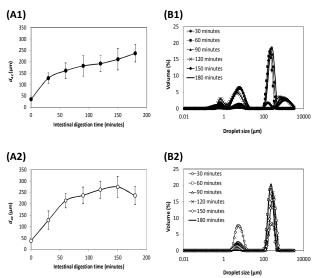
Figure 7. Mean droplet size (A) and distribution (B) of WPM (closed symbols) and HT WPM-stabilized emulsions (open symbols) as a function of time in presence of simulated intestinal fluid (containing bile salts and pancreatin).
