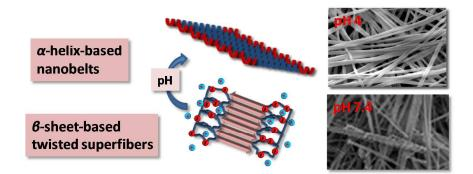
**Figure 8.** Schematic representation of the hierarchicaly self-assembled Pala<sub>5</sub>-PGA<sub>11</sub>-Pala<sub>5</sub> triblock copolypeptide at different pH. In the left, SEM images of the discovered structures after freeze drying of the peptide aqueous hydrogel formulations. Inspired from reference 112.
