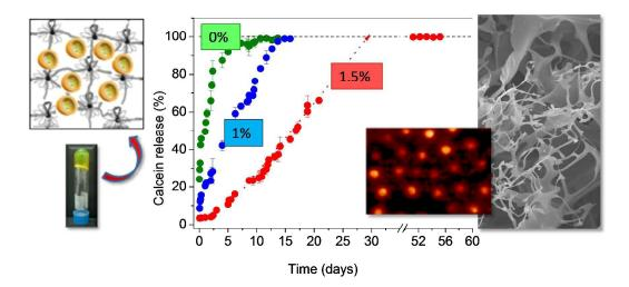
**Figure 1.** Sustained calcein release at physiological pH through the liposome/hydrogel formulation (left schematic representation) at different gelator concentration. In the right, SEM and AFM images of the involved hydrogel. Inspired from references 20 and 21.
