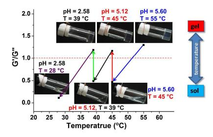
**Figure 2.** pH tunable thermo-responsiveness of a hydrogel formed by self-assembly of a ABA triblock copolymer composed of poly(ethylene oxide) (PEO) end-capped by poly(methoxydi(ethylene glycol) methacrylate-*co*-methacrylic acid) pH/thermo-sensitive outer blocks. Reprinted with permission from *Langmuir*, 26, 8787-8796 (ref 27) Copyright 2010, American Chemical Society.
