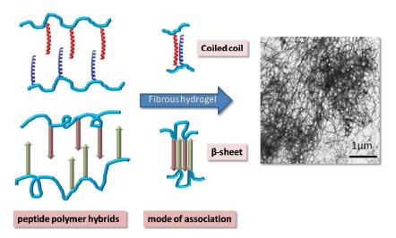
**Figure 4.** Schematic representation of the self-assembly of graft copolymers hybrids (PHC type) through the formation of either coiled coil or  $\beta$ -sheet motifs that leads to fibrous hydrogels (cryoTEM image). Inspired from references 70 and 71.
