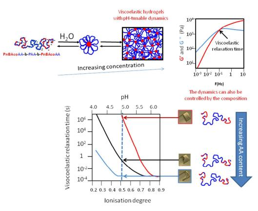
**Figure 3.** Influence of composition of the end-blocks of P(AA-*co*-nBA)-*b*-PAA-*b*-P(AA-*co*-nBA) aqueous solutions as a function of degree of ionization of the AA moieties controlled by pH. Inspired from references 46 and 49.
