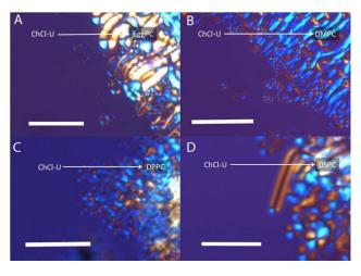
Figure 2. Polarizing optical microscopy images of phospholipids (A: EggPC, B: DMPC, C: DPPC, D: DSPC) with choline chloride-urea (ChCl-U) DES, showing vesicle formation above their transition temperatures (Table 1). Scale bars =  $50\mu m$ .
