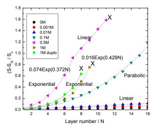
Figure 2. Reflectometry-signal values at the end of each build-up cycle as functions of layer number, at various ionic strengths from 0 to 1M. "X" indicates the occurrence of instability and the end of the build-up process. The 1M duplo is for a repeated experiment on a different oxidized-silicon substrate, and using slightly different exposure durations.
