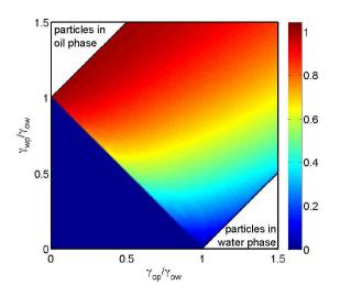
FIG. 3: The ratio of rigid-particle over perfectly-soft-particle adsorption energies for particles adsorbing from water onto an oil-water interface. The adsorption energy depends sensitively on surface tensions when  $\gamma_{wp}/\gamma_{ow} \ll 1$  and  $\gamma_{op}/\gamma_{ow} \approx 1$ .
