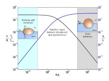
FIG. 5: The scaling of contact-line displacements shows the transition from perfectly-soft to rigid behaviour of particles. The black curve shows ridge height  $u_r(R, \pi/2)$ scaled by  $R\gamma_{ow}/\gamma_p$ . This plateaus for  $R \leq 0.1L$  where
