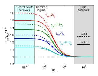
FIG. 6: The adsorption energy of soft particles normalised by the adsorption energy of a rigid particle for various values of  $\gamma_p/\gamma_{ow}$ . Dashed/continuous curves correspond to  $\nu = 0.4/0.5$  respectively. Large particles with  $R > 10^3 L$  appear rigid. Small particles with R < 0.1L have a constant adsorption energy, equivalent
