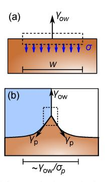
FIG. 7: Deformation of a plastic surface by a contact line. (a) Control volume on an initially flat solid surface where surface tension,  $\gamma_{ow}$ , is balanced by an average bulk stress,  $\sigma$ , over a region of size w. (b) Deep within the plastic region, indicated by the dashed box, the equilibrium ridge shape is determined by a Neumann balance between solid surface tension  $\gamma_p$  and  $\gamma_{ow}$ .
