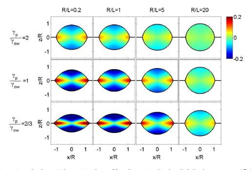
FIG. 4: Deformation of soft particles at interfaces. Non-dimensionalised radial displacements  $u_r/R$  for a range of R/L and  $\gamma_p/\gamma_{ow}$ . Particles only show large-scale deformations when their radius is small compared to the elastocapillary length, L. For  $R \ll L$ , particles adopt a fixed, lenticular shape given by Neumann's construction.
