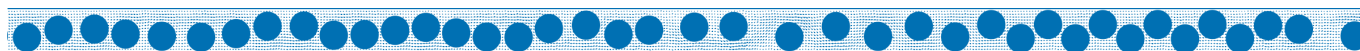
Fig. 17 Simulation snapshot illustrating the formation of ordered and unordered subregions within a train of 40 droplets. The right part of the train has ‘frozen’ into a stable zigzag configuration, while the left part exhibits a travelling sine-wave. †
