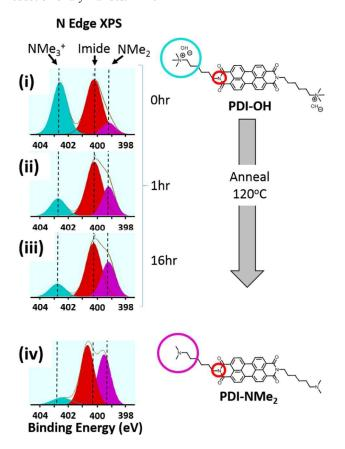
**Figure 2.** Conversion of  $NMe_3^+$  to  $NMe_2$  in PDI-OH proceeds upon thin film annealing at 120 °C (i-o hrs, ii-1 hr, iii-16 hrs) as observed via XPS (N 1s spectra). As expected, after extended annealing, the
