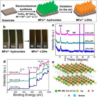
Fig. 1 (a) Scheme of the synthetic route to MFe-LDH (M= Co, Ni and Li) nanoarrays; (b) photograph of MFe-LDH nanoarrays growing on the Ni foam before and after self-oxidation in the air; (c) XRD patterns and (d) XPS spectra of MFe-LDH (M= Ni, Co and Li) nanoplatelet arrays; (e) structure model of MFe-LDH.
