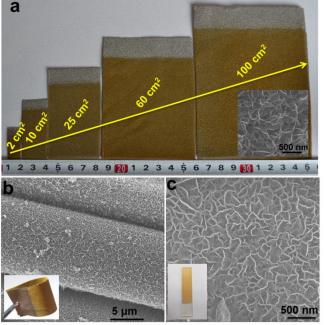
**Fig. 5** (a) Photographs of NiFe-LDH nanoplatelet arrays synthesized on the foam nickel substrates with various scales (inset: the SEM image of NiFe-LDH on 100 cm<sup>2</sup> substrate): synthesis time for all the samples is 300 s at room temperature. SEM images for NiFe-LDH nanoplatelet arrays on (b) the conducting cloth and (c) FTO substrate (inset: their corresponding photographs).
