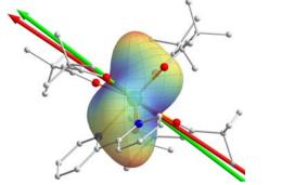
**Fig. 4** Magnetic principal axes, determined experimentally (red arrow) and calculated from the electrostatic potential (green arrow). As can be seen by the surface representation of the calculated relative potential energy, where blue is lowest and red is highest, the easy axis is oriented along the lowest potential energy direction.
