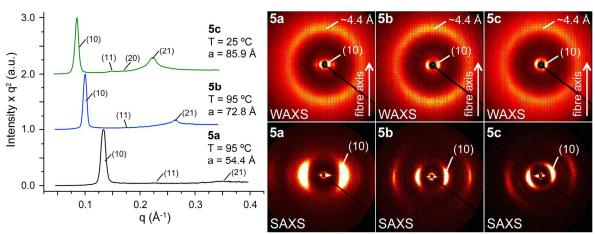
Fig. 2 Left: representative small-angle powder diffraction plots of **5a–c** collected in the hexagonal columnar ( $\Phi_h$ ) phase (collection temperature, diffraction peaks and dimension are indicated). Right: Wide- (WAXS) and small- (SAXS) angle X-ray diffraction patterns collected for oriented fibres of **5a–c** in the  $\Phi_h$  phase at 25 °C.
