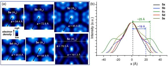
Fig. 3 (a) Comparison of the relative electron density distributions calculated from the smallangle powder diffraction data shown in Figs. 2 and S19–20. (b) Relative electronic density profiles of the columnar hexagonal ( $\Phi_h$ ) phases (the estimated distance between the centre of the column and the spacer are indicated).
