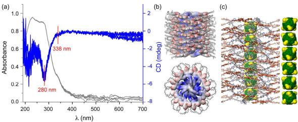
**Fig. 5** CD/UV spectra measured from the spin coated film of **5d** in the temperature range of 30–70 °C (a), molecular model of the supramolecular column (b) and detail of the core region (c). In (a) the two negative Cotton effects observed at 280 and 338 nm, respectively, are indicated.
