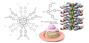
[60]Fullerene dendronized with 12 chiral or achiral self-assembling dendrons forms discs with fullerene at their centre that self-organise into helical columns with a fullerene nanowire-like core.
