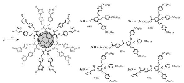
Scheme 3 Synthesis of compounds 5a-e. *Reagents and conditions*: a) 4a-e, TBAF, CuSO<sub>4</sub>•5H<sub>2</sub>O, sodium ascorbate, CH<sub>2</sub>Cl<sub>2</sub>/H<sub>2</sub>O (5a: 64%, 5b: 85%, 5c: 89%, 5d: 63%, 5e: 62%).
