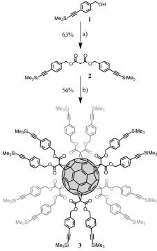
Scheme 1 Synthesis of compound 3. *Reagents and conditions*: a) malonyl chloride, pyridine,  $CH_2Cl_2$ , 0 °C to RT, 16 h (63%); b)  $C_{60}$ , DBU,  $CBr_4$ , *o*-DCB, RT, 72 h (56%).
