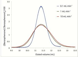
**Figure 3** Dispersion of a 10  $\mu$ L sample plug of benzophenone in MeCN ([Benzophenone]<sub>0</sub> = 1.015 × 10<sup>-2</sup> M) through coiled stainless steel tubing of 1 mm internal diameter and 10 mL capacity at 30 °C and the flow rates indicated. Concentrations were obtained by UV absorbance.
