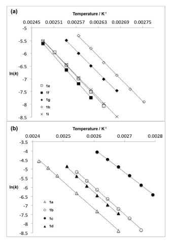
Figure 6 Arrhenius plots for thermal decomposition of (a) 1,3-dioxin-4-ones **1e-i** with different 6-position substituent  $R^1$  and (b) 1,3-dioxin-4-ones **1a-d** with different 2-position substituent  $R^2$ .
