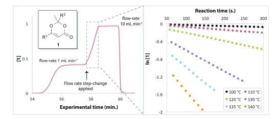
Rapid acquisition of kinetic data for thermolysis of 1,3-dioxin-4-ones is demonstrated with a commercial meso-scale flow reactor, using a step-change in flow rate or 'push-out' from the flow line. 175x75mm (300 x 300 DPI)
