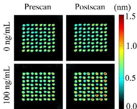
**Figure 3** Protein spot mass profile (protein layer height in units of nm) of each well derived from the reflectance map. (Adapted from *Biosens Bioelectron.*, 2011, 26, 1871-1875).
