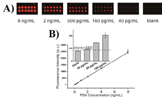
**Figure 10** A) Microscopic fluorescence images of DNA tetrahedron-based microarrays for PSA assay, B) Linear calibration curve of PSA assay (Inset: Histogram showing the LOD of PSA assay).
