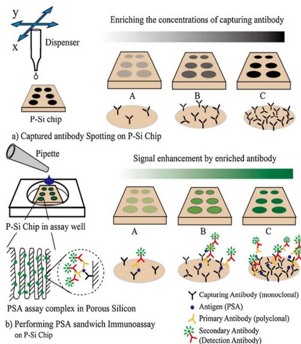
**Figure 14** Fabrication and application of P-Si chip for PSA detection. (a) By increasing the concentration of cAb the surface density of the spotted cAb can be increased. (b) Higher density of cAb microarray allows enhanced signal readouts. (Adapted from *Anal Chim Acta*. 2013, 796, 108-14).
