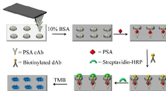
**Figure 7** Schematic representation of the PSA assay development. (Adapted from *Anal. Chem.* 2013, 85, 5617–5621).
