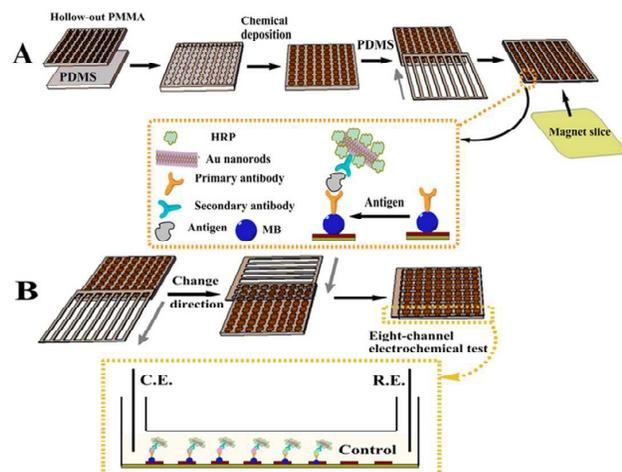
**Figure 8** (A) Preparation of the flexible microchip and the construction of multiplexed immunoassay interface; (B) Sketch map of eight spots in one microchannel in detection of three antigens for prostate cancer. (Adapted from *ACS Appl. Mater. Interfaces* 2014, 6, 20137–20143).
