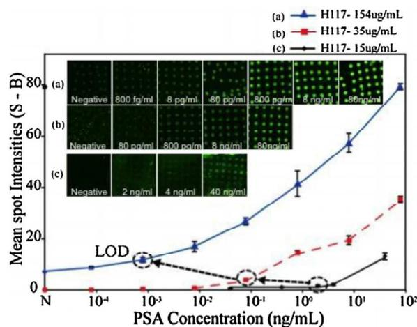
**Figure 15** Effect of increased concentration of immobilized cAb on the PSA detection sensitivity of P-Si protein microarray. (Adapted from *Anal Chim Acta*. 2013, 796, 108-14).
