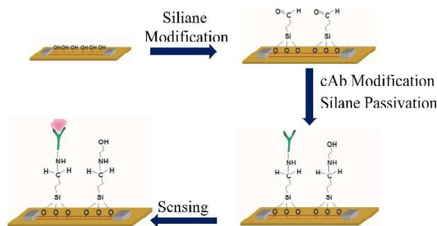
**Figure 4** Antibody modification at SiNW surface, including: silane modification, antibody modification, silane passivation and sensing steps.
