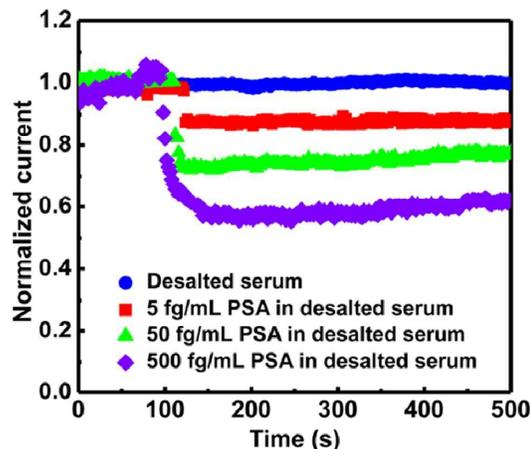
**Figure 5** Normalized current with respect to various PSA concentrations in desalted human serum. Desalted serum without PSA exhibited no electrical response. (Adapted from *Anal. Chem.*, 2013, 85, 7912–7918).
