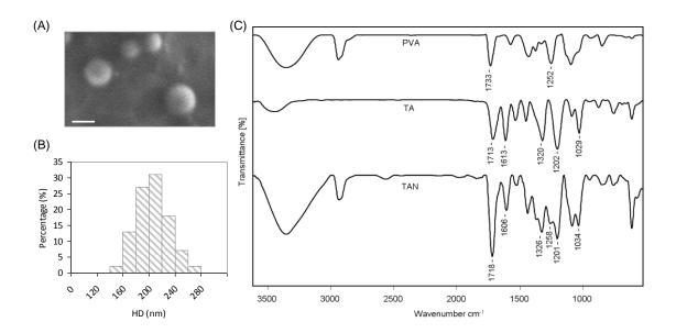
Fig. 3 Tannic acid nanoparticles characterization. (A) SEM image of TA nanoparticles (scale bar 100 nm). (B) Hydrodynamic diameter of TA nanoparticles. (C) FTIR spectra of PVA, TA and TA nanoparticles.
