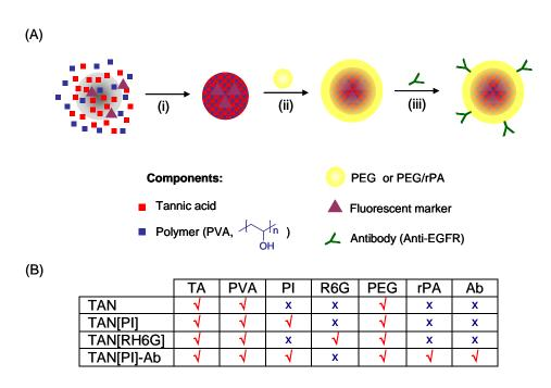
Fig. 2 (A) Schematic representation of nanoparticle fabrication. Synthesis of TA nanoparticles (i). In this step the addition to the reaction medium of a fluorescent marker (optional) allows the fabrication of fluorescent-TA nanoparticles. Nanoparticles were then coated with PEG, or a mixture of PEG and rProtein A (ii) to allow the conjugation to a targeting antibody (iii). (B) Composition of nanoparticles used in this study.
