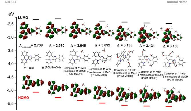
Figure 8. Frontier MO of 11 and complexes of 11 with MeOH (DFT B3LYP/6-31+G(d,p), PCM for MeOH).
