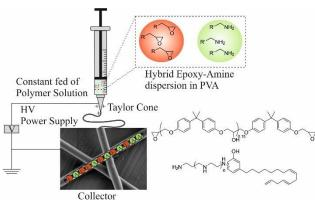
Fig.1 Schematic representation of the colloid electrospinning process and the statistical distribution of the epoxy and amine compartments in the obtained nanofibres on basis of the PVA-EA 3:1 sample. PVA serves as matrix polymer which keeps the reactive colloidal domains separated. Furthermore, the simplified chemical structures of the epoxy and amine are displayed.
