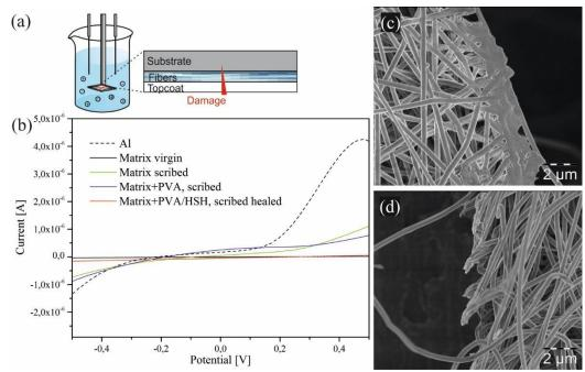
Fig. 6 Self-healing ability of the PVA-EA 3:1 sample. a) Schematic drawing of the setup for the voltammetry measurements. b) Current versus Potential curves comparing the virgin coating (black), the pure Al-foil (black, dashed) with the scribed non-healing (green and blue) and the self-healing coating (red). SEM image of the scribed c) PVA-EA sample versus d) the scribed PVA nanofibres.
