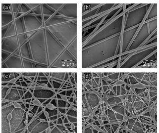
Fig. 2 SEM images of the dual compartment (PVA-EA) fibres with different matrix to colloid ratios a) 6:1 b) 3:1 c) 2:1 d) 1:1.
