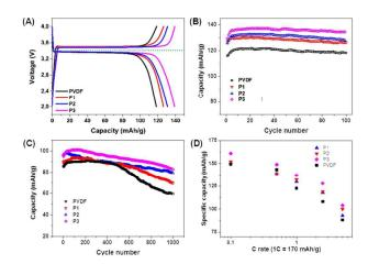
**Fig. 2** Electrochemical properties of LiFePO $_4$  electrodes using different PIL binders. (A) Charge-discharge curves at a current density of 1C (= 170 mA/g). (B) Cycling performance up to 100 cycles at 1C. (C) Cycling performance up to 1000 cycles at 5C (= 850 mA/g). (D) Rate capability for PIL binders and PVDF. The rate capability data of PVDF (the black line in Fig. a, B and C) was taken from ref. 29. (active materials loading 2.5mg)
