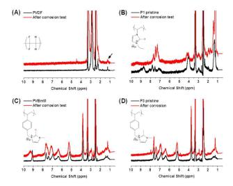
**Fig. 3** <sup>1</sup>H-NMR spectra of PVDF and 3 PIL binders to track changes of the chemical structure before and after the electrochemical corrosion test. (A) PVDF, (B) P1, (C) P2 and (D) P3. The black arrow in a point out a peak assigned to a grease residue involved in all samples.
