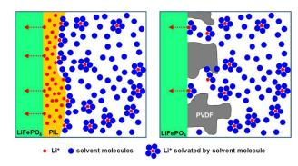
**Fig. 5** Hypothetic schematic illustration of effect on PIL/electrolyte heterophase for high Li<sup>+</sup> conductivity (left). On the other hand, PVDF blocks the Li<sup>+</sup> transport (right), therefore, it shows a higher resistance (=low Li<sup>+</sup> flux) compared to the cathode composed with the PIL binders. For the simplification, carbon additives are not described in the figure.
