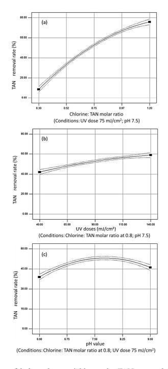
Figure 2 The effects of independent variable on the TAN removal in the chlorine/UV process. (a) Chlorine: TAN molar ratio; (b) UV doses; (c) pH value. Experimental condition:  $[TAN]_0= 0.07 \text{ mmol/L}$ ; 0.01 mol/L phosphate buffer
