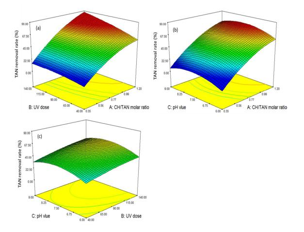
Figure 3 Response surfaces plotted on the effects of two independent variables on the TAN removal in the chlorine/UV process. (a) Chlorine: TAN molar ratio and UV dose; (b) Chlorine: TAN molar ratio and pH; (c) UV dose and pH. Experimental condition:  $[TAN]_0= 0.07 \text{ mmol/L}; 0.01 \text{ mol/L} phosphate buffer$
