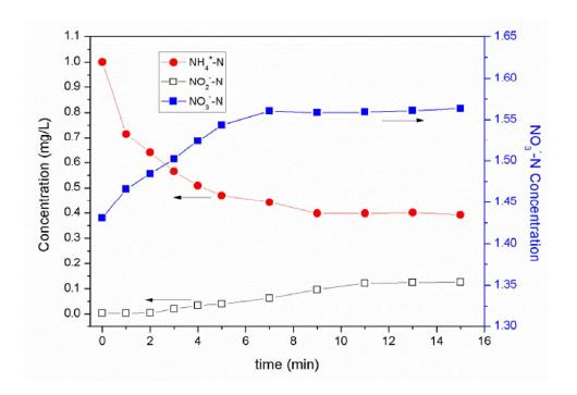
Figure 4 Nitrogenous products for TAN decomposition in the UV/chlorine process with
