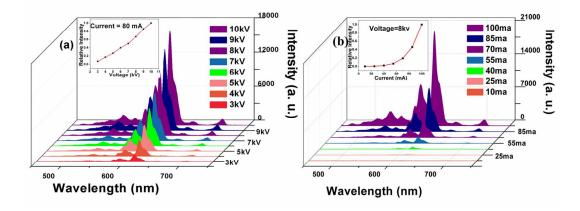
Fig.7 Cathodoluminescence properties of  $NaLa_9(GeO_4)_6O_2:0.07Eu^{3+}$  (a) with a constant filament current 80 mA ( the inset shows the voltage related CL intensity) and (b) under a constant voltage 8.0kV (the inset shows the current related CL intensity).
