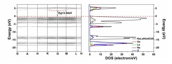
Fig. 3 Calculated band structures (left) and DOS (right) of hexagonal  $NaLa_9(GeO_4)6O_2$  near the Fermi energy level (the red dash below). The Fermi energy is the zero of the energy scale. Eg is the calculated forbidden band gap of the ground
