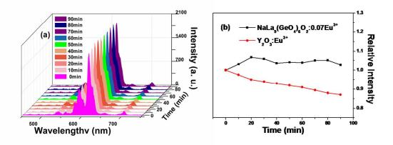
Fig. 8 (a) Degradation property of  $NaLa_9(GeO_4)_6O_2:0.07Eu^{3+}$  and (b) time dependence intensity compared with
