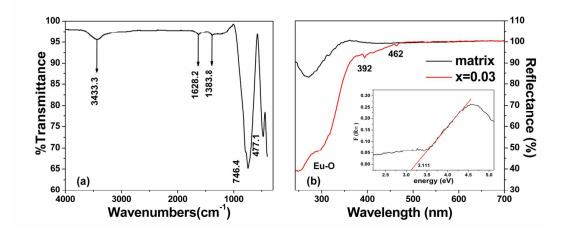
Fig. 2 (a) FITR spectrum of  $NaLa_9(GeO_4)_6O_2$ , and (b) DRS of the matrix and  $NaLa_9(GeO_4)_6O_2$ : 0.07Eu<sup>3+</sup>, the inset
