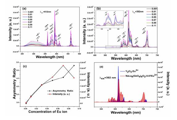
Fig. 4 (a) The PLE spectra of samples with Eu<sup>3+</sup> concentrations from 0.001 to 0.11; (b) PL spectra of all the samples
