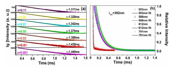
Fig. 6 (a) Decay curves of different concentrations of  $Eu^{3+}$  (from 0.001 to 0.11) doped samples when excited at 392 nm and (b) 0.07  $Eu^{3+}$  doped sample monitoring under different wavelength of 553, 588, 612, 701 nm when excited at 392 nm.
