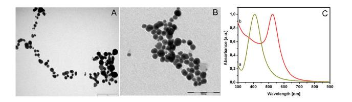
**Fig. 1** Transmission Electron Micrographs of: (A) NPs-CM and (B) AgNPs-CM. (C) Normalized absorption spectra of: (a) AgNPs-CM and (b) AuNPs-CM
