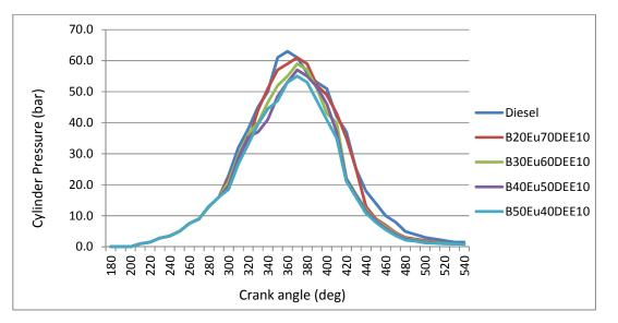
Fig 11: Variation of crank angle with cylinder pressure
