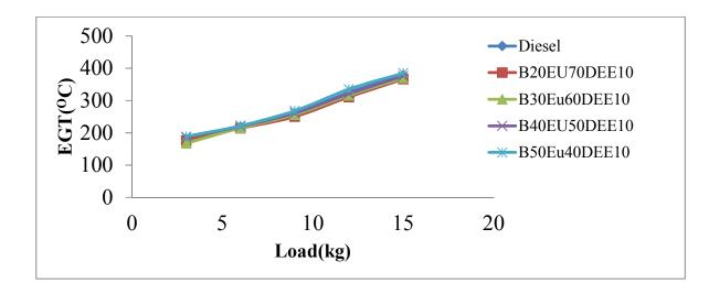
Fig.5. Variation of exhaust gas temperature versus load
