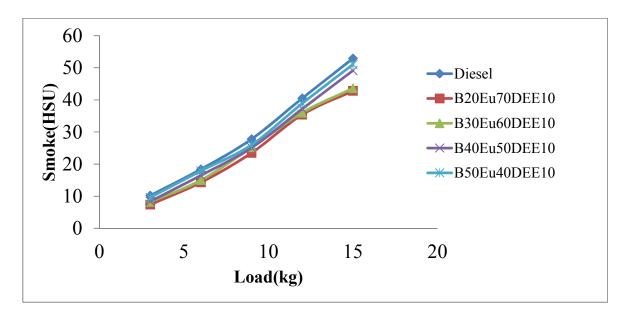
Fig.9. Variation of smoke emission versus load
