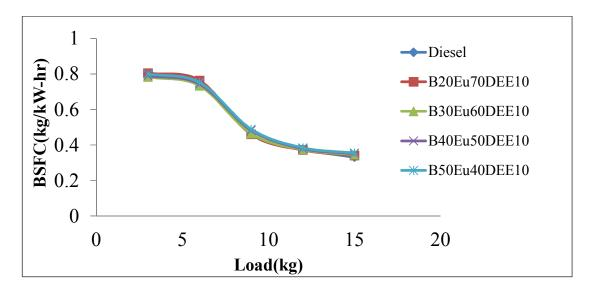
Fig.3. variation of Brake specific Fuel consumption versus load
