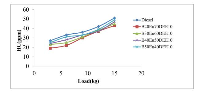
Fig.7. Variation of hydrocarbon emission versus load
