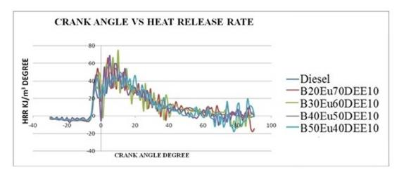
Fig 10: Variation of crank angle with heat release rate
