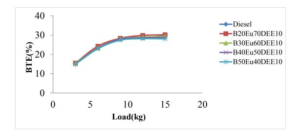
Fig.4. Variation of brake thermal efficiency versus load
