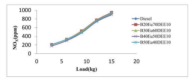
Fig.8. Variation of oxides of nitrogen emission versus load
