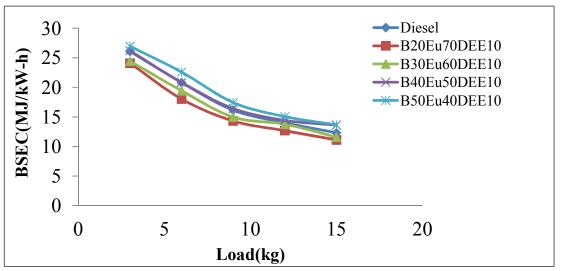
Fig.2. variation of Brake specific energy consumption versus load
