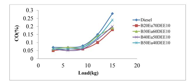
Fig.6. Variation of carbon monoxide emission versus load
