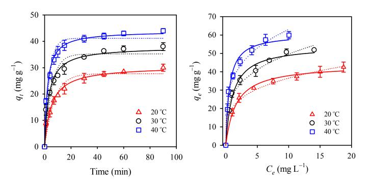
Fig. 5. Effect of temperature on (a) the adsorption kinetics and (b) adsorption isotherm.
