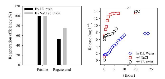
Fig. 7. Effect of regeneration methods on (a) recyclability and (b) desorption behavior of diclofenac from CTAB-ZIF-67 at 30 °C.
