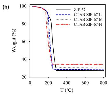
Fig. 3. Effects of CTAB loading on (a) surface charge and (b) thermal stability of CTAB-ZIF-67.
