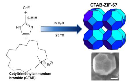
Fig. 1. Schematic illustration of the synthesis of ZIF-67 functionalized with CTAB (scale bar in the SEM image is 200 nm).
