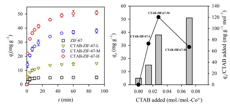
Fig. 4. Effect of CTAB loading on (a) the adsorption kinetics and (b) qe/mol-CTAB at 30 °C.
