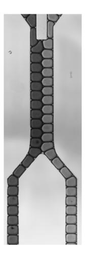
**Figure 6**: Splitting a stream of synchronized droplets in an A-B alternate configuration into its constituent droplets and recombination of the separated streams. Direction of flow is from top to bottom (indicated by the arrow). This produces a situation where a uniform of droplets are flowing through the individual channel, but where each side contains droplets of different composition.
