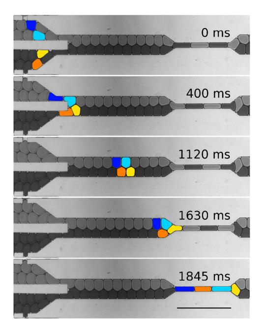
**Figure 2**: A series of images extracted from a high-speed video (Movie S1) showing a set of droplets moving through the synchronization architecture (scale bar -  $600 \mu m$ ). Droplets are passively ordered into an A-B alternating pattern when they are injected into the common channel (400 ms into the video). Once this channel is constricted so as to only allow a single file of droplets (1600 ms into the video) the two rows of droplets are impelled into an A-B sequential order.
