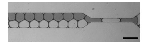
**Figure 4**: Synchronization of droplets with diameters of up to 150 um (scale bar - 300  $\mu$ m). Application of vacuum to the output allows for more accurate and faster synchronization. The device shown is a directly scaled up version of the previously described design.
