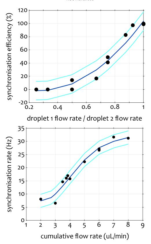
**Figure 5**: (a) Dependence of synchronization performance on droplet size difference. A synchronization efficiency above 95% is only achieved if the two synchronized droplet types enter the chamber at equal flow rates. (b) Dependence of the synchronization rate on total flow rate, showing that throughput increases as a function of flow rate.
