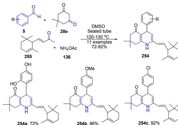
**Scheme 96.** Catalyst free synthesis of substituted 7,8-dihydroquinolin-5-(1H,4H,6H)-ones **254**; some representative examples are shown.
