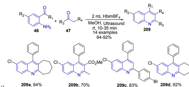
**Scheme 75.** Synthesis of substituted quinolines **209** in ionic liquid under ultra-sound irradiation; some representative examples are shown.
