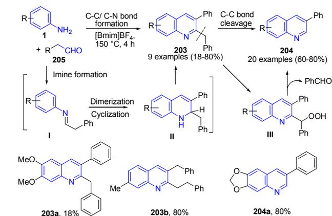
**Scheme 72.** Synthesis of 2,3-disubstituted **203** and 3-substituted quinolines **204** in ionic liquid; some representative examples are shown.
