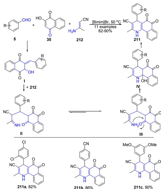
**Scheme 77.** Synthesis of polysubstituted benzo[h]quinolines **211** in ionic liquid; some representative examples are shown.
