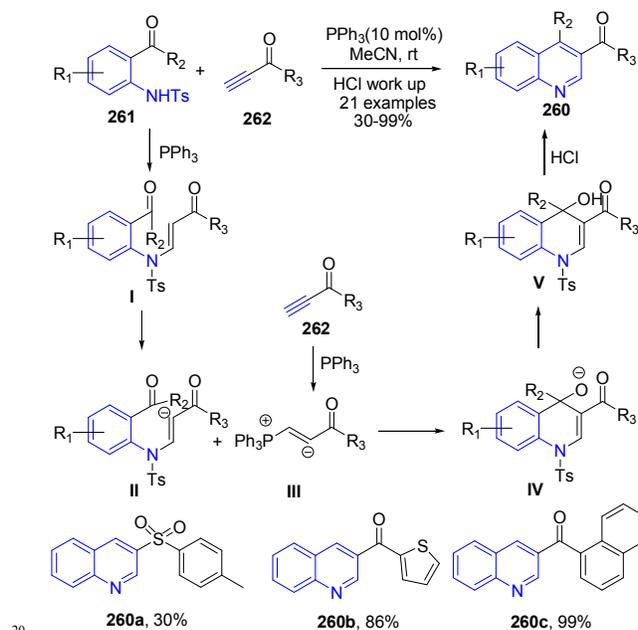
**Scheme 99.** Phosphine-catalyzed synthesis of dihydroquinolines **260**; some representative examples are shown.
