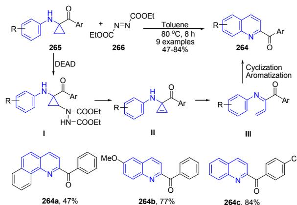
**Scheme 101.** Catalyst free synthesis of 2-benzoyl quinolines **264** from 1,1-cyclopropane aminoketones **265**; some representative examples are shown.
