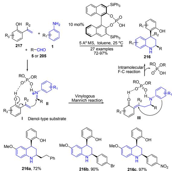
**Scheme 80.** Chiral phosphoric acid-catalyzed synthesis of cis-disubstituted tetrahydroquinolines **216**; some representative examples are shown.
