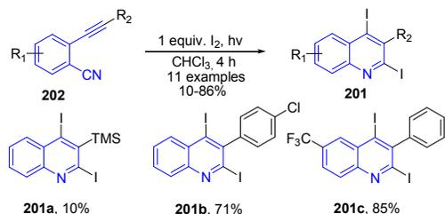
**Scheme 71.** Synthesis of 2,4-diiodoquinolines **201** via the photochemical cyclization of *o*-alkynylaryl isocyanides **202** with molecular iodine; some representative examples are shown.
