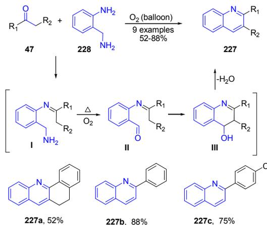
**Scheme 86.** Catalyst-free synthesis of 2-substituted quinolines **227** by treatment of 2-(aminomethyl)aniline **228** with ketones **47**; some representative examples are shown.
