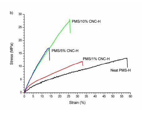
Typical tensile stress versus strain curves registered at room temperature of low Young's modulus PMS and PMS/CNC nanocomposites cured under low crosslinking conditions (L) from mannitol/sebacic mannitol/sebacic acid rate 1:2 (a). Typical tensile stress versus strain curves registered at room temperature of high Young's modulus PMS and PMS/CNC nanocomposites cured under high crosslinking conditions (H) from mannitol/sebacic acid rate 1:2 (b).
