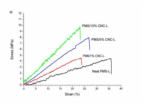
Typical tensile stress versus strain curves registered at room temperature of low Young's modulus PMS and PMS/CNC nanocomposites cured under low crosslinking conditions (L) from mannitol/sebacic mannitol/sebacic acid rate 1:2 (a). Typical tensile stress versus strain curves registered at room temperature of high Young's modulus PMS and PMS/CNC nanocomposites cured under high crosslinking conditions (H) from mannitol/sebacic acid rate 1:2 (b).
