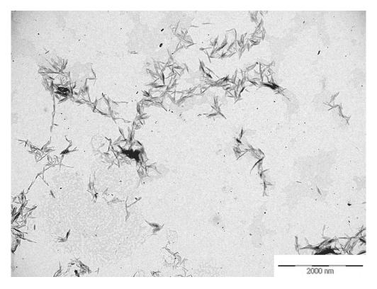
Transmission electron micrograph (TEM) of CNC isolated by hydrolysis with sulfuric acid. 233x174mm (150 x 150 DPI)
