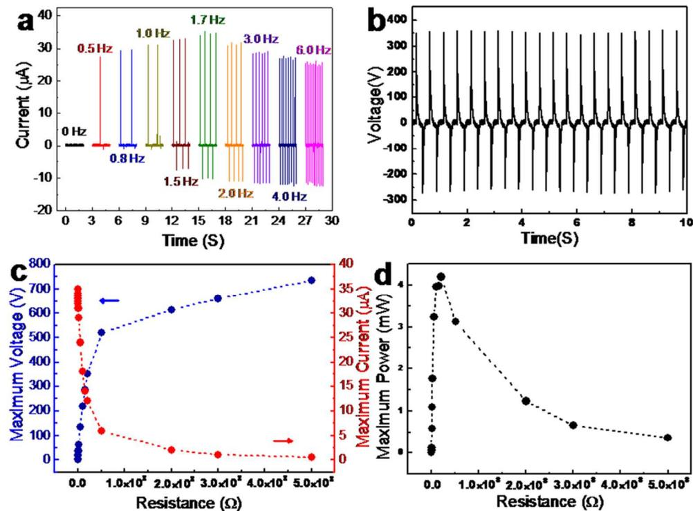
(a) The output current of the PDMS/Ag/ZnO/PDMS NG under the frequency of a value from 0 Hz to 6 Hz. (b) The open-circuit voltage of the PDMS/Ag/ZnO/PDMS NG. (c) The plots of output voltage and current versus external loads. (d) The output power corresponding to the external loads.
