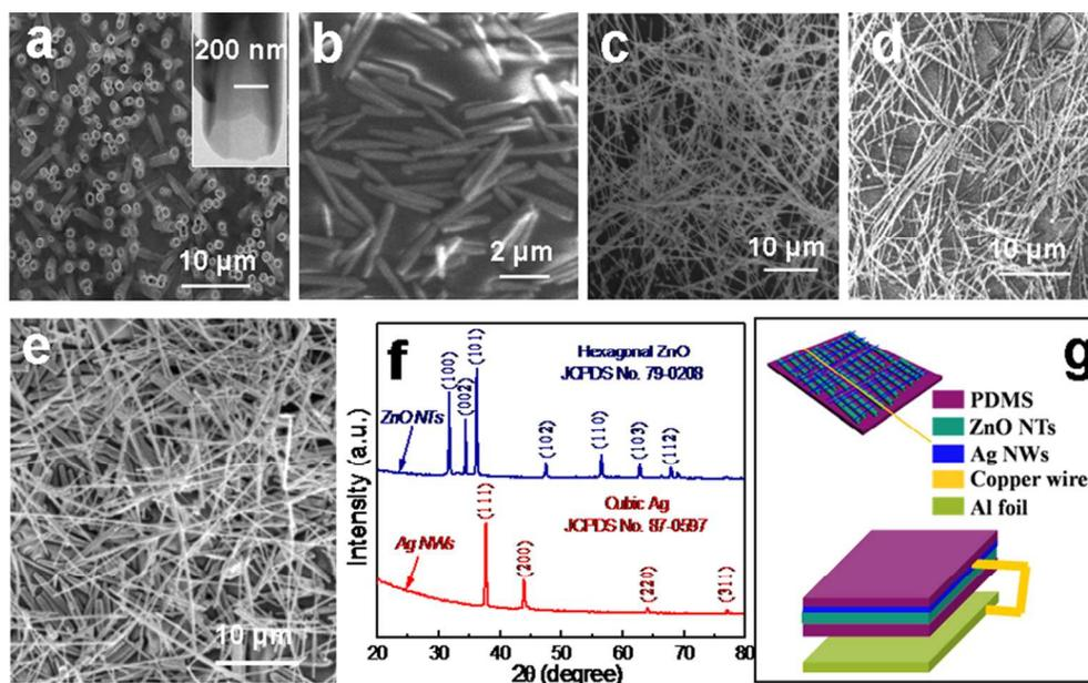
SEM image of (a) ZnO NTs, (b) ZnO NTs aligned laterally on the surface of PDMS matrix, (c) the synthesized Ag NWs, (d) Ag NWs deposited on the surface of PDMS matrix and (e) Ag NWs deposited on ZnO NTs aligned laterally on the surface of PDMS matrix. (f) XRD patterns of ZnO NTs and Ag NWs. (g) The structure diagram of composite PDMS based NG.
