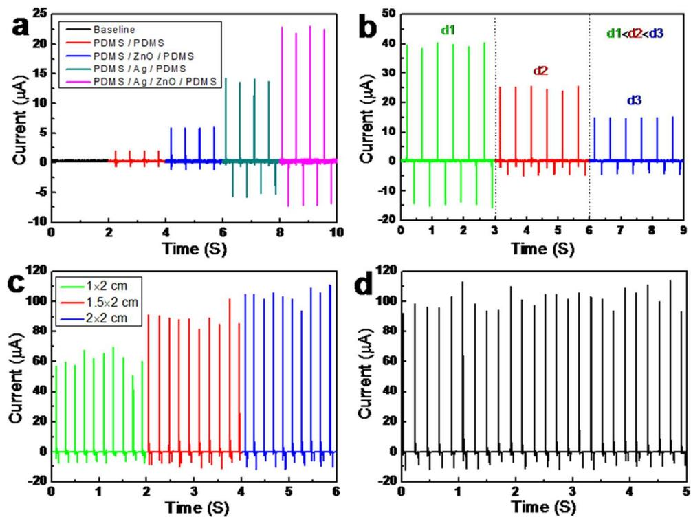
The output current of (a) four kinds of nanogenerator based on different structure, (b) three PDMS/Ag/ZnO/PDMS NGs with different PDMS thickness under periodic external stress (20 N). (c) The maximum output current of three PDMS/Ag/ZnO/PDMS NGs with different sizes. (d) The maximum output current of PDMS/Ag/ZnO/PDMS NG.
