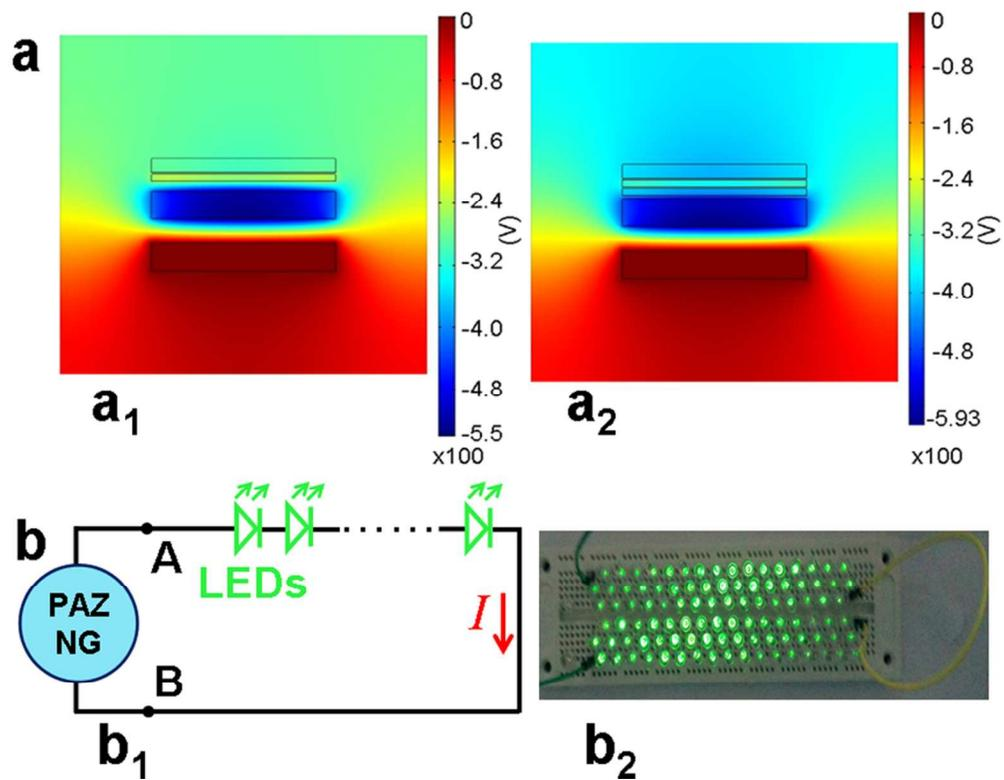
The potential distribution in (a1) PDMS/Ag/PDMS NG and (a2) PDMS/Ag/ZnO/PDMS. (b) A circuit diagram (b<sub>1</sub>) and a photograph of 99 green LEDs (b<sub>2</sub>) that are directly powered by the NG. 85x65mm (300 x 300 DPI)
