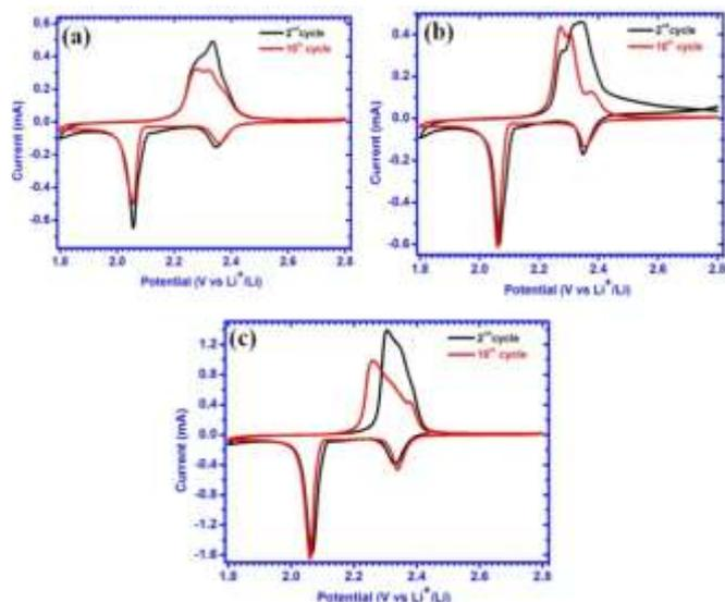
**Fig. 8** Second and tenth CV cycle behavior of (a) SCAC-50 (b) SCAC-60 and (c) SCAC-66 composite cathode recorded at a scan rate of 0.1 mV/s
