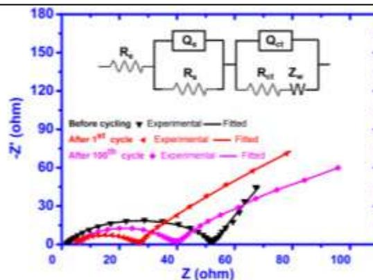
**Fig. 10** Experimental and fitted Impedance spectra of the as fabricated cell containing SCAC-60 cathode and the cell after completing 1 and 100 cycles (Inset- corresponding equivalent circuit).
