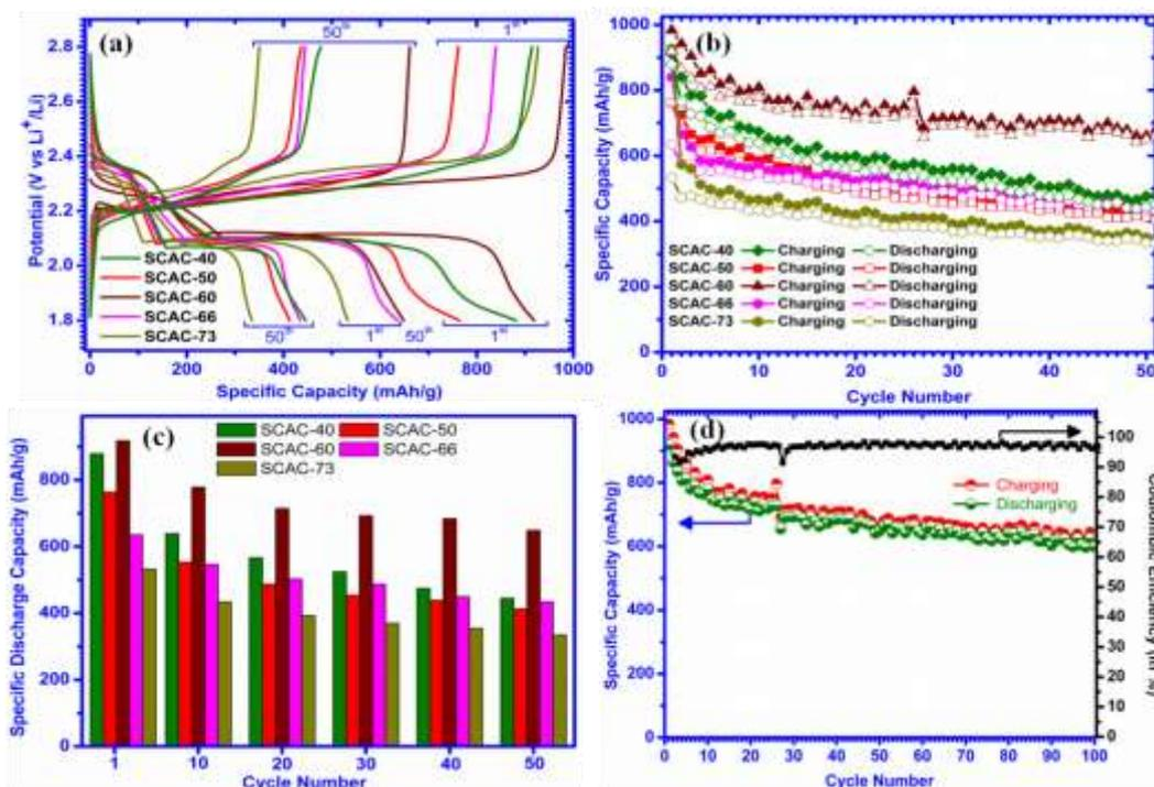
**Fig. 9** (a) Comparative galvanostatic charge/discharge (b) cycle life (c) selective cycle life behavior of all sulfur-loaded carbon aerogel composites under a current rate of C/10 and (d) extended cycle life study of SCAC-60 cathode
