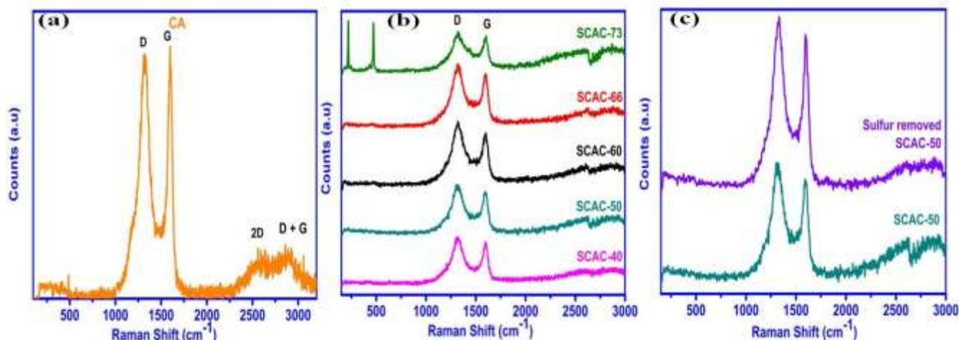
**Fig. 3** Raman spectrum of (a) carbon aerogel, (b) sulfur-carbon aerogel composites and (c) 50 wt. % sulfur loaded and sulfur removed carbon aerogel composites.
