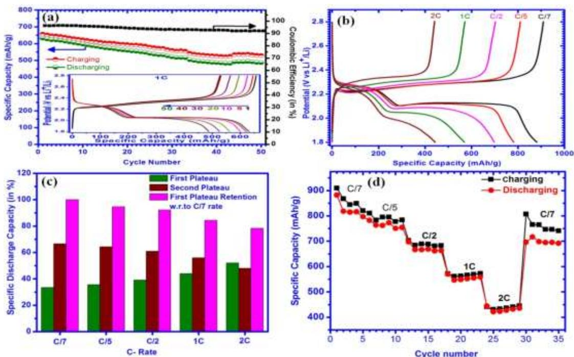
**Fig. 11** (a) High (1C) rate cycling behavior (inset- selective discharge/charge curves) (b) discharge/charge curves (c) retention of discharge plateaus and (d) cycling and retention behavior of SCAC-60 cathode under the influence of different current rates.
