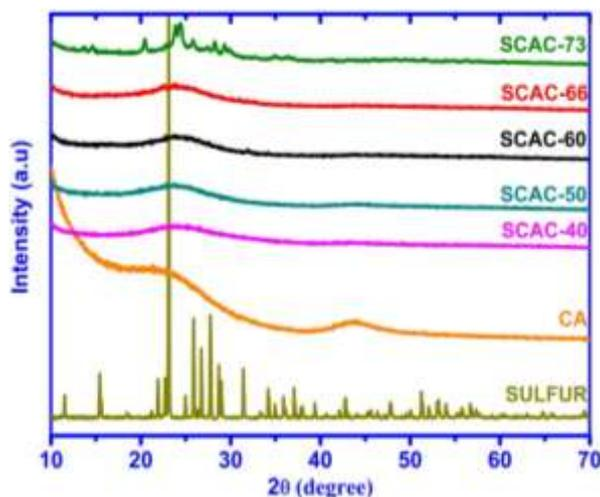
**Fig. 1** XRD pattern of sulfur, carbon aerogel, 40 wt. %(SCAC-40), 50 wt. %(SCAC-50), 60 wt. %(SCAC-60), 66 wt. %(SCAC-66) and 73 wt. %(SCAC-73) sulfur loaded carbon aerogel.
