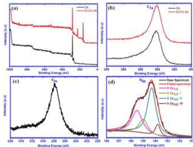
**Fig. 7** (a) Survey spectra, (b) 1s carbon spectra of CA and SCAC-60 and (c) and (d) correspond to 2s and 2p spectra containing fitted photoelectron lines of sulfur in SCAC-60 respectively.
