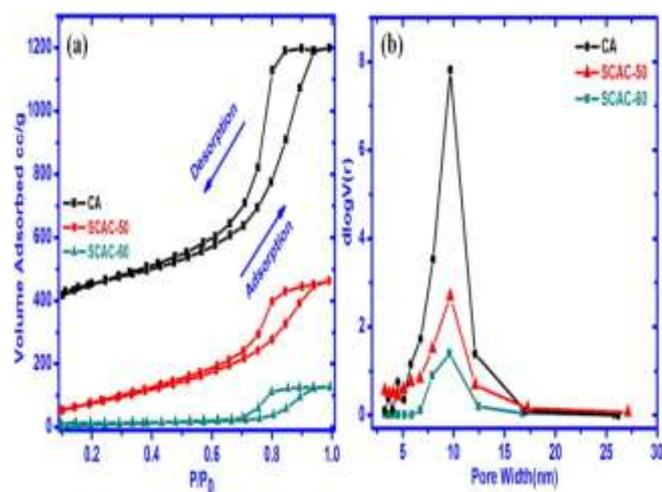
**Fig. 4** (a) Nitrogen adsorption-desorption isotherm of carbon aerogel and select sulfur-carbon aerogel composites and (b) corresponding pore volume distribution.
