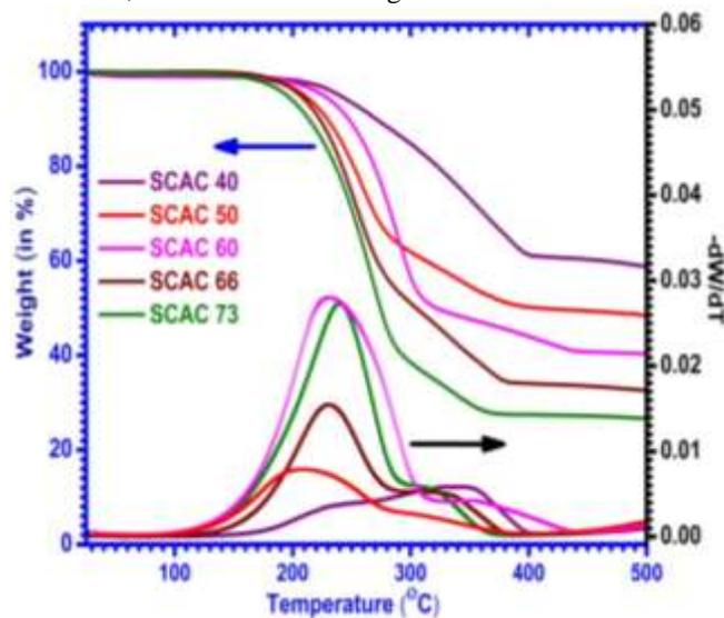
**Fig. 2** Thermogravimetry analysis of sulfur-carbon aerogel composites.
