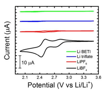
**Figure 1**. Cyclic voltammograms of 5 mM 2,3,6-TMQ in various 0.2 M Li-ion salt/PC electrolytes. All experiments were performed in a GC / Li / Li cell at a scan rate of 10 mV/s.
