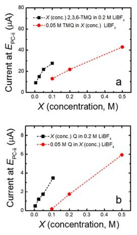
**Figure 2.** Peak reduction current of the  $2^{nd}$  wave of 2,3,6-TMQ (a) and quinoxaline (b) as a function of either active species and LiBF<sub>4</sub> concentration. In all experiments, PC was used as a solvent. Peak currents were obtained from CV measurements taken in a GC / Pt / Ag/Ag<sup>+</sup> cell at a scan rate of 10 mV/s.
