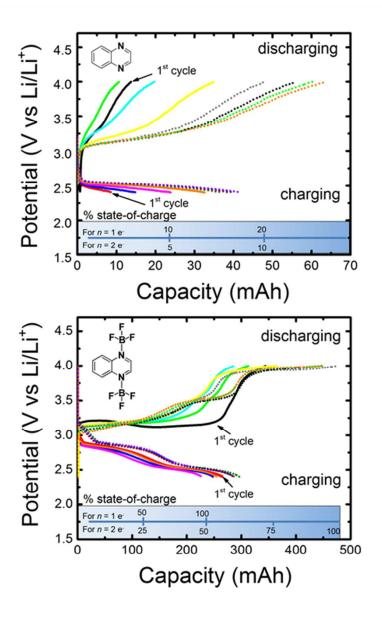
**Figure 7**. Capacity curves from the constant-current chronopotentiometry bulk electrolysis cycling of 5 mM quinoxaline in 0.2 M LiBF<sub>4</sub> / PC (top) and 5 mM 2(BF<sub>3</sub>)Q in 0.2 M Li triflate / PC (bottom). The charging and discharging current was 5 mA. 8 charge-discharge cycles are shown, with dotted lines representing the last 4 cycles.
