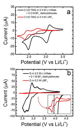
**Figure 3**. Effects of adding BF<sub>3</sub>, in the form of BF<sub>3</sub>•OEt<sub>2</sub>, on the redox activity of (a) 5 mM 2,3,6-TMQ, and (b) 5 mM quinoxaline at scan rates of 10 mV/s and 20 mV/s, respectively.
