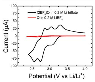
**Figure 6.** Cyclic voltammetry of 5 mM quinoxaline (bis)trifluoroborane ((2BF<sub>3</sub>)Q) and 5 mM quinoxaline (Q) in 0.2 M Li triflate / PC and 0.2 M LiBF<sub>4</sub> / PC respectively. Experiments were performed at a 20 mV/s scan rate.
