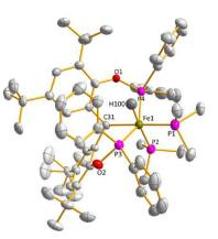
**Figure 3**. ORTEP plot of complex **2** at the 50% probability level (hydrogen atoms except for Fe–H are omitted for clarity). Selected bond lengths (Å) and angles (deg): Fe1-P4 2.141(1), Fe1-P3 2.142(1), Fe1-C31 2.165(3), Fe1-P1 2.231(1), Fe1-P2 2.269(1), Fe1-H100 1.50(3); C31-Fe1-P1 177.67(9), P2-Fe1-H100 170(1), P4-Fe1-C31 81.74(9), P3-Fe1-C31 81.99(9).
