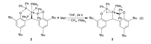
The reaction of 2 with iodomethane afforded an unsaturated coordinated complex 3 as red crystals with the release of a methane molecule (eq. (2)) in the yield of 87%.
