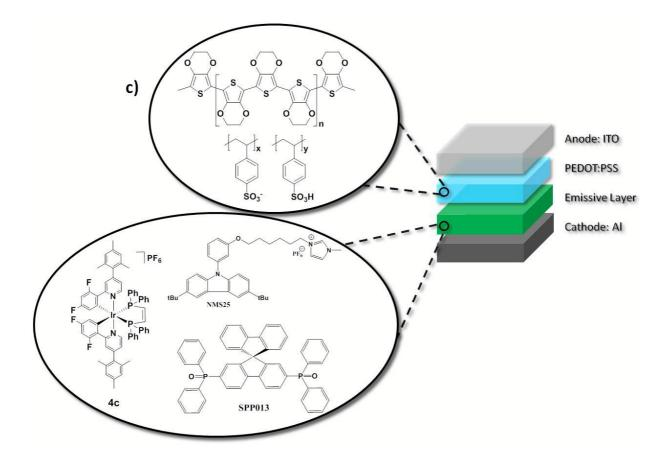
Figure 7. a) and b) Luminance (solid blue line) and average voltage (open red squares) for ITO/ PEDOT:PSS / Active layer /Al (Active layer = 1:1 by mass of NMS25:SPPO13 with 10 wt.% of 4c) with a pulsed driving regime (block-wave pulsed current; 1000 Hz; 50 % duty cycle; average density 100 A m<sup>-2</sup>). c) Schematic representation of the LEEC architecture.
