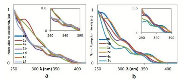
Figure 5. UV-Vis spectra of complexes 1a, 2a, 4a, 1b, 1d, 1e, 1f (a) and 2b, 4b, 1c, 2c, 4c, 3c (b) recorded in MeCN at 298 K.
