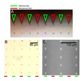
**Fig. 4.** Sequence-selective binding of zfRC-LH1 to matched and mismatched dsDNA using dual-sequence DPN. **(a)** DNA printing using pens to create alternate 5 µm spots of matched (green) and mismatched (red) DNA. **(b)** Bright field image of the printed DNA array. **(c)** Fluorescence image of the pattern after ZF-RC-LH1 binding to DNA. Each row is spaced 66µm apart. Excitation: 532 nm. Emission: > 650 nm.
