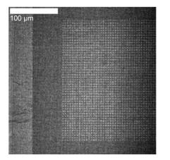
**Fig. 3.** Fluorescence microscopy image of zfRC-LH1 binding to DNA-functionalized glass surfaces. The DNA was patterned in a regular array of 2  $\mu$ m squares, defined by electron-beam lithography. Excitation: 532 nm. Emission: > 650 nm. The fluorescence signal on the left of the picture relates to a large marker in order to aid array location.
