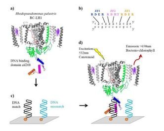
**Fig. 1. (a)** Structure of the RC-LH1 from *Rhodopseudomonas palustris* (grey) with the Hsubunit highlighted in green (structure adapted from ref. 5). **(b)** An eleven bp DNA *zif268* recognition sequence. **(c)** Immobilization of cyclooctyne-tagged dsDNA to an azide-modified surface. **(d)** Excitation Energy Transfer (EET) was measured between the carotenoid pigment (in red) and bacteriochlorophyll (highlighted in purple) as a test for photosynthetic function.
