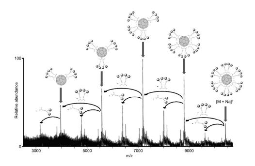
Figure 4. MALDI-ToF mass spectrum of compound  $C_{60}(E)_{12}$ . The typical fragments of retro-Bingel reaction and hydrolysis of a malonic ester followed by decarboxylation can be attributed.
