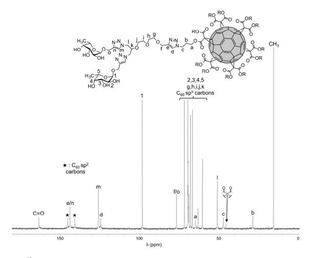
Figure 3. <sup>13</sup>C NMR spectra of  $C_{60}(E)_{12}$  recorded in  $D_2O$  (100 MHz, 20°C).
