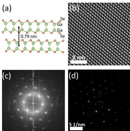
**Figure 1** Few-layered GaSe crystal structure and its TEM images. (a) Layered crystal structure of GaSe with each tetra-layer (TL) formed by Se-Ga-Ga-Se atomic sheets. (b) High resolution TEM images from few-layer GaSe. Fast Fourier Transforms (c) and SAED pattern (d).
