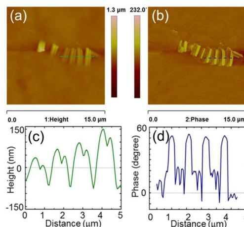
**Figure 2** Atomic force microscopy measurements on wrinkled GaSe sheets a. AFM topography and b. AFM phase mode images of few-layer wrinkled GaSe. c-d. The corresponding height profiles of sheets shown in a, b.
