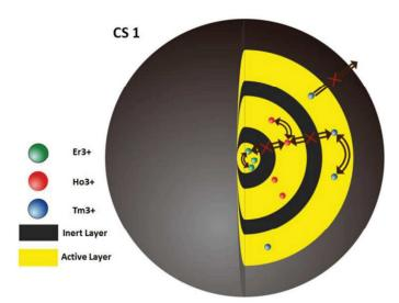
Fig. 17. Multilayered design with inert sub-layers to reduce cross-relaxation between activators: NaYF<sub>4</sub>:Er(10mol%)@NaYF<sub>4</sub>@NaYF<sub>4</sub>:Ho(10mol%)@NaYF<sub>4</sub>@NaYF<sub>4</sub>:Tm(1mol%)@NaYF<sub>4</sub>. Reprinted with permission from Shao et al<sup>189</sup>. Copyright 2014, Wiley-VCH Verlag GmbH & Co. KGaA.
