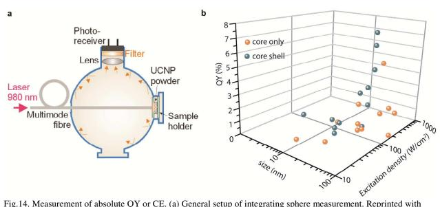
Fig.14. Measurement of absolute QY or CE. (a) General setup of integrating sphere measurement. Reprinted with permission from Zhao et al.<sup>46</sup>. Copyright 2013, Nature Publishing Group. (b) Reported literature values for absolute QY as a dependency of size and  $I_{ex}$  from table 2, excluding values from ref.<sup>42</sup>.
