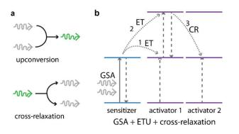
Fig. 4. (a) Schematic illustration of the energy transfer (ET) in upconversion and cross-relaxation (CR) processes and energy level diagram (b) of the ETU process followed by deleterious cross-relaxation, quenching the radiative energy level of activator 1.
