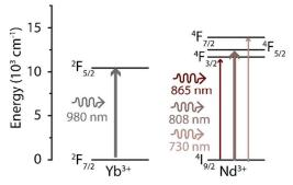
Fig. 13. Schematics of the energy levels taking part in GSA by two commonly used sensitizers, Yb<sup>3+</sup> and Nd<sup>3+</sup>.
