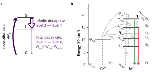
Fig. 5. (a) Schematic representation of simple 3-level model described in Section 4.1. (b) Main radiative and nonradiative transistions and energy transfer processes relevant for UCL in a NaYF<sub>4</sub>:Yb,Er nanocrystal, described in section 4.2. The energy levels relevant in the rate equations are denoted Yb<sub>1,2</sub> and Er<sub>1-6</sub>. Reproduced from Zhao *et al.*<sup>46</sup> with permission from The Royal Society of Chemistry.
