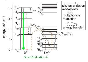
Fig. 9. Co-doping Er3+ with Sm3+ in NaYF<sub>4</sub> crystals results in a green/red emission ratio of 4, due to quenching of the red emitting states of  $\text{Er}^{3+}$  by Sm<sup>3+</sup>. Reproduced from Chan *et al.*<sup>42</sup>. Copyright (2012) American Chemical Society. We made a minor correction by inserting the (brown) energy transfer arrows for the Er  ${}^{4}I_{13/2} \rightarrow \text{Sm}^{\,6}F_{3/2}$   ${}^{6}H_{15/2}$   ${}^{6}F_{1/2}$  transition for completeness.
