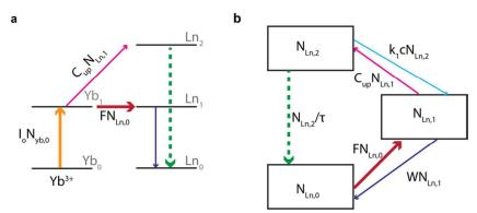
Fig. 6. (a) Energy spacing and energy transfer between different states of sensitizer Yb and the activator Ln-ion. (b) Schematic diagram of the key energy transfer processes represented in the rate equations (24)-(27). Rectangles represent state populations. Reproduced with permission from Zhao et al.<sup>25</sup>, copyright 2013, Nature Publishing Group.
