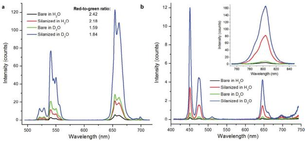
Fig. 16. By measuring the UCL in  $H_2O$  and  $D_2O$  the effects of surface quenching by OH-groups can be quantified as shown in (a) for NaYF<sub>4</sub>:Yb,Er UCNPs and in (b) for NaYF<sub>4</sub>:Yb,Tm UCNPs, both bare and silanized. Reproduced from Arppe et al. ref.<sup>182</sup> with permission from The Royal Society of Chemistry.
