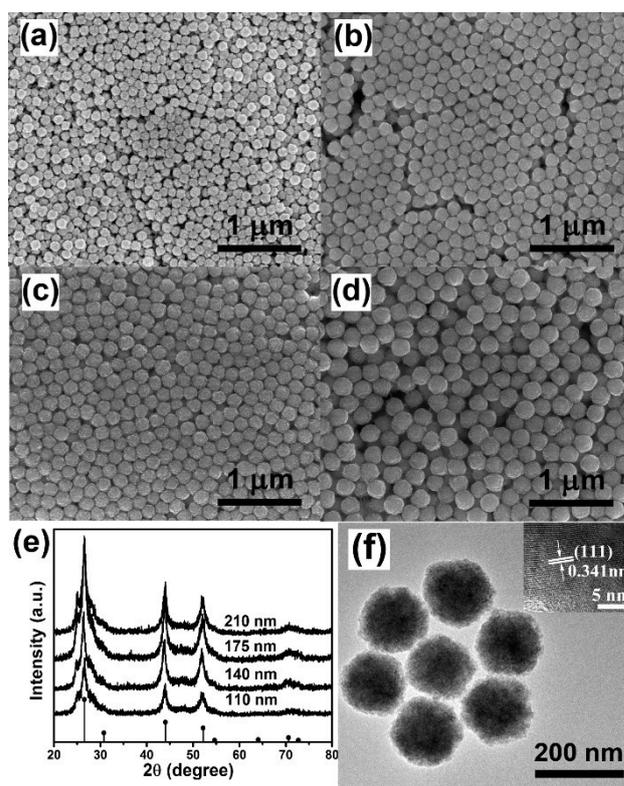
**Figure 3** (a-d) SEM images of CdS spheres with different amount of Cd precursor for further growth. (a) 2 mmol, 110 nm; (b) 4 mmol, 140 nm; (c) 5 mmol, 175 nm; (d) 6 mmol, 210 nm; The molar ratio of Cd and TU was kept 1:1 in all experiments; (e) XRD patterns of CdS products with different diameters; (f) TEM image of typical products (inset: HR-TEM image of a CdS sphere showing the nanocrystalline domains)
