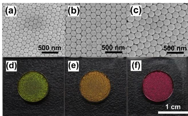
**Figure 4.** SEM images of photonic crystal films with  $\text{Cu}_2\text{O}$  spheres in different diameters as building blocks: (a) 133 nm; (b) 165 nm; (c) 187 nm; (d-f) digital photograph of  $\text{Cu}_2\text{O}$  photonic crystal films fabricated in PMMA template with  $\text{Cu}_2\text{O}$  spheres in diameter of 133 nm, 165 nm and 187 nm respectively.
