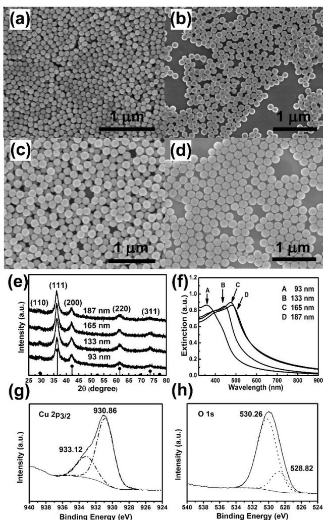
**Figure 2** SEM images of  $\text{Cu}_2\text{O}$  spheres with different amount of Cu precursor. (a) 0.4 mL; (b) 0.6 mL; (c) 0.8 mL; (d) 1 mL; The diameters (a-d) are  $93 \pm 7$  nm,  $133 \pm 10$  nm,  $165 \pm 10$  nm,  $187 \pm 13$  nm respectively. (e) XRD patterns of  $\text{Cu}_2\text{O}$  products with different diameters; (f) Extinction spectra of the  $\text{Cu}_2\text{O}$  spheres in different diameters; (g-h) XPS spectrum of  $\text{Cu}_2\text{O}$  spheres in diameter of 133 nm
