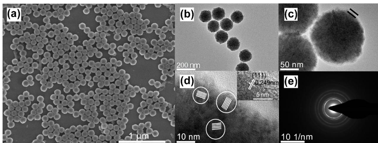
**Figure 1** Images of a typical synthesis product with 0.6 mL Cu precursor added. (a) SEM image; (b-d) TEM images with different magnification times; (e) SAED image
