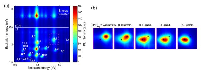
Figure 2: (a) PLE map of a completely functionalized HiPCO solution. (b) Zoom on the region highlighted by a dashed red rectangle in (a) for selected TPP concentrations illustrating the evolution of the coverage of the (6,5) species. The black stars point at the shifted (resp. unshifted) position of the lines for a fully functionalized (resp. unfunctionalized) sample.
