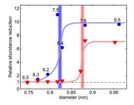
Figure 4: Relative reduction of the resonant PL intensity of different species, between a stock HiPCO solution and the same solution after partial functionalization followed by a 5 hour centrifugation (120000 g). Two different monomers concentrations (1  $\mu$ mol.L<sup>-1</sup>, red or 3  $\mu$ mol.L<sup>-1</sup>, blue) give different diameter selectivity. The vertical lines highlight the cut-off diameter for each TPP concentration.
