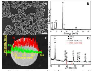
Figure 1. (A) SEM image, (B) EDX Spectrum of the  $TiO_2/Pt$  Janus submicromotors; (C) linear EDX analysis of Pt and Ti over a typical TiO2/Pt submicromotor; (D) XRD pattern of the  $TiO_2/Pt$  Janus submicromotors.
