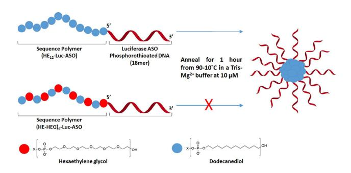
**Figure 1 - Precision polymers conjugated to antisense oligonucleotides (ASO)**. (Top) ASO polymer with 12 dodecane (C12) repeat units self-assembles into micelles in aqueous media. (Bottom) ASO polymer with an alternating sequence of hexaethylene glycol-dodecane units does not assemble into micelles in aqueous media.
