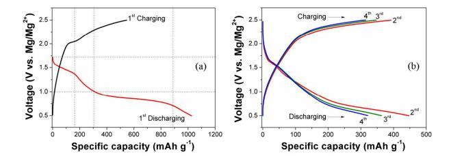
Fig. 8: (a) Initial and (b) 2<sup>nd</sup>, 3<sup>rd</sup> and 4<sup>th</sup> charge-discharge curves of S-*rGO* nanocomposite at a current density of 20 mA g<sup>-1</sup> in the voltage range of 0.5-2.5 V vs. Mg/Mg<sup>2+</sup>.
