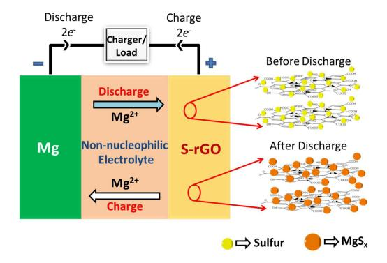
Fig. 10: (a) Electrochemical mechanism of S-rGO nanocomposite electrode within Mg/S cell.
