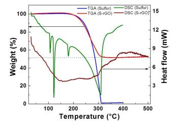
Fig. 4: TGA-DSC analysis of sulfur and S-rGO nanocomposite under 20 ml/min helium flow and 10 °C/min heating rate.
