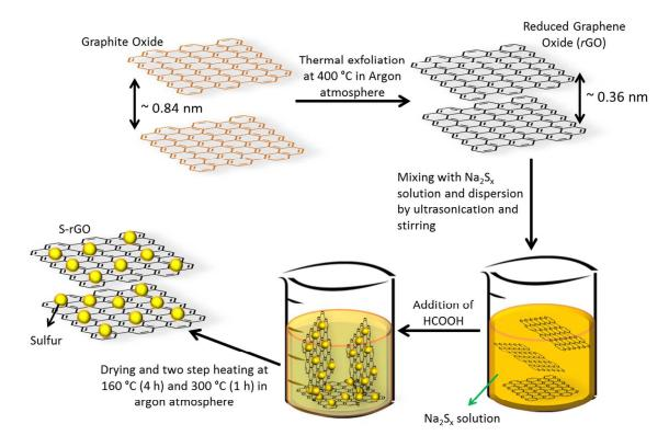
Fig. 1: Schematic diagram of the synthesis procedure adopted for synthesizing graphene based sulfur nanocomposite.
