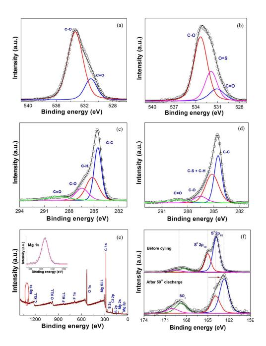
Fig. 7: (a, b) High resolution O1s XPS spectra of *rGO* and S-*rGO*. (c, d) High resolution C1s XPS spectra of *rGO* and S-*rGO*. (e) XPS survey spectrum of S-*rGO* cathode after 50 battery cycles in the discharge state. Inset shows the high resolution Mg 1s XPS spectrum. (f) Comparison of high resolution S2p XPS spectra of S-*rGO* cathode electrode before battery cycling and after 50 cycles in the discharge state.
