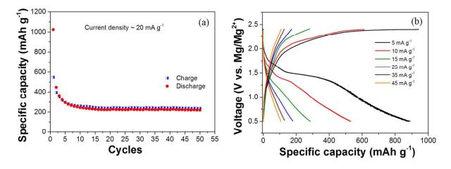
Fig. 9: (a) Cyclic stability of S-rGO nanocomposite for the initial 50 cycles at the current density of 20 mA  $g^{-1}$ . (b) Current rate capability of S-rGO electrode for current densities between 5 and 45 mA  $g^{-1}$ .
