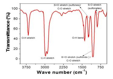
Fig. 5: FTIR spectrum of S-rGO nanocomposite.
