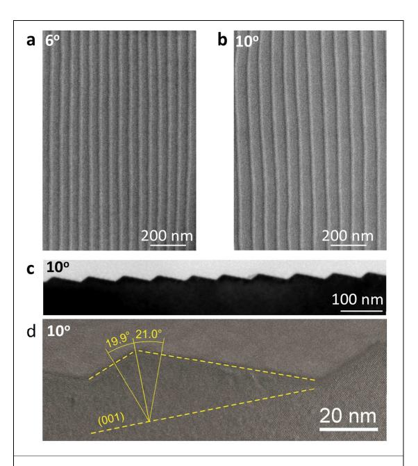
**Figure 3. Ordered, asymmetric nanogroove patterns formed on ion irradiated GaAs(001) surfaces with miscut. a**, SEM image of nanogroove structures formed on GaAs (001) with a miscut of 6° and **b**, with a miscut of 10° towards [110] direction, respectively. **c-d**, Cross-sectional TEM images of the nanogroove patterns. The facet angles with respect to the GaAs (001) plane are indicated.
