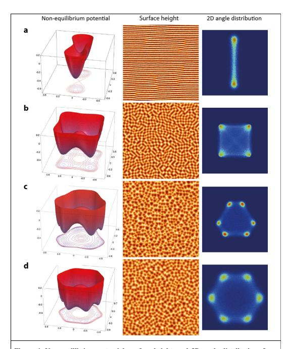
Figure 4. Non-equilibrium potential, surface height, and 2D angle distributions from numerical integrations of the continuum equation for reverse epitaxy. Non-equilibrium potentials have been chosen to have minima at slopes  $(m_x, m_y)$  corresponding to the facet angles and symmetries with **a**, two-fold (GaAs(001)), **b** four-fold (Ge(001)), **c** three-fold (Ge(111)), and **d** six-fold (Si(111)) symmetry, respectively.
