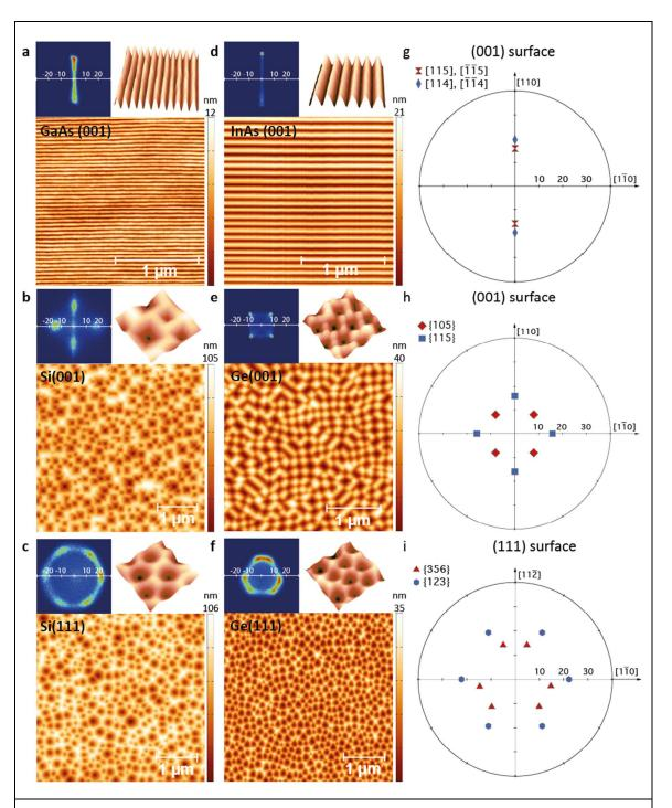
**Figure 2.** Atomic Force Microscopy images of nano-patterns fabricated by ion irradiation on the surfaces of different semiconductors. (a) nanogrooves on GaAs(001), (b) inverse squared pyramids on Si(001), (c) inverse hexagonal pyramids on Si(111), (d) nanogrooves on InAs(001), (e) inverse squared pyramids on Ge(001), and (f) inverse pyramids on Ge(111), respectively. The two-dimensional angle distribution (left) covering an area of  $\pm 30^{\circ}$  and the
