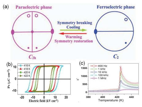
**Figure 2.** (a) Schematic figure of the order-disorder phase transition. (b) Ferroelectric hysteresis loops of diisopropylammonium bromide under different temperature. (c) Temperature dependent dielectric constant under different frequencies. Reproduced from reference<sup>50</sup> with the permission of American Association for the Advancement of Science.
