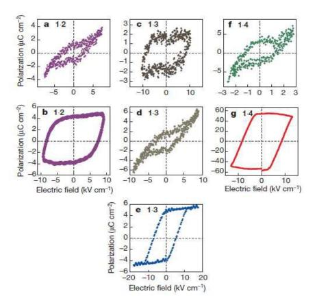
**Figure 4.** (a) and (b) are the polarization versus electric field curves for LASO complexes 1.2 at 300 K and 74 K. Complex 1.3 at 300 K (c, d) and 7 K (e), and complex 1.4 at 300 K (f) and 7 K (g). Reproduced from reference<sup>35</sup> with the permission of Nature Publishing Group.
