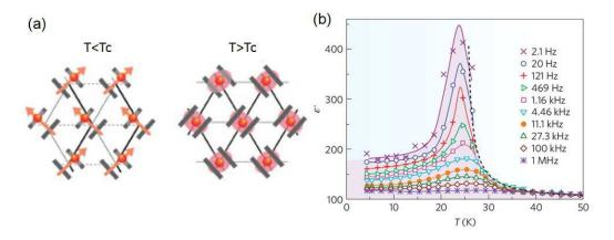
**Figure 7.** (a) Schematic drawings for temperatures below and above Tc of organic charge-transfer salt  $\kappa$ -(BEDT-TTF)<sub>2</sub>Cu[N(CN)<sub>2</sub>]Cl. (b) Temperature dependent dielectric constant under different frequency. Reproduced from reference<sup>42</sup> with the permission of Nature Publishing Group.
