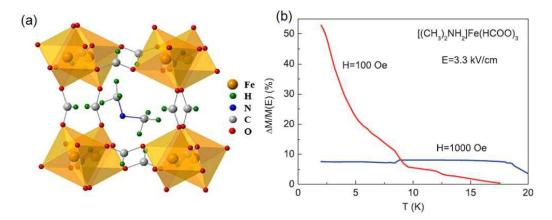
**Figure 8.** (a) Molecule structure of Fe-MOF. (b) tunability of magnetization by electric field. Reproduced from reference  $^{43}$  with permission of Wiley-VCH.
