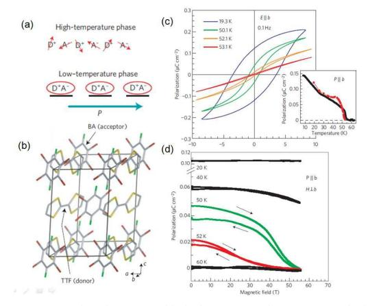
**Figure 5.** (a) Schematic structure of ionic donor (TTF) and acceptor (BA) mixed stacks in high and low temperature. P denotes electric polarization. (b) Crystal structure of TTF–BA. (c) P-E loops of TTF-BA under different temperature, the inset shows temperature dependent polarization. (d) The tunability of polarization by magnetic field. Reproduced from reference<sup>41</sup> with the permission of Nature Publishing Group.
