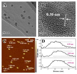
**Fig. 1** Characterizations for the monolayer-NiTi-LDH nanosheets. A) TEM image; B) HRTEM image; C) AFM image and D) the corresponding height profiles; the numbers from 1 to 3 in (D) correspond to the numbers from 1 to 3 in (C).
