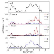
Fig. 4 Total DOS (TDOS) and Partial DOS (PDOS) of  $\mathrm{Ni}^{3+}$  doped monolayer-NiTi-LDH.
