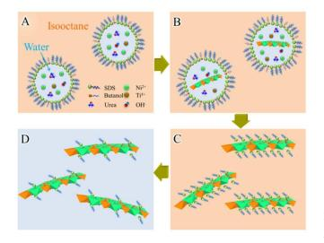
Scheme 1 Schematic representation for the formation of monolayer-NiTi-LDH nanosheets in micelle: (A) metal salts and urea mix in water droplets; (B) LDH starts to form during the hydrolysis of urea; (C) the monolayer-NiTi-LDH nanosheets form in isooctane; (D) monolayer-NiTi-LDH nanosheets are transferred into water surrounding after cleaning.
