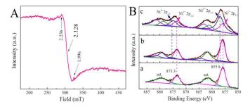
**Fig. 3** (A) EPR spectrum of as-prepared monolayer-NiTi-LDH at 110 K under Ar atmosphere. (B) Ni 2p XPS spectra of (a) bulk-NiAl-LDH, (b) bulk-NiTi-LDH and (c) monolayer-NiTi-LDH.
