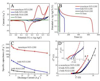
Fig. 2 (A) CV curves; (B) galvanostatic discharge curves; (C) current density dependent on the specific capacitance; and (D) Nyquist plots of EIS for monolayer-NiTi-LDH, bulk-NiTi-LDH and bulk-NiAl-LDH.
