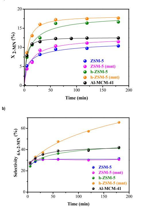
**Figure 7.** Acylation of 2-methoxynaphthalene. Evolution along the reaction time of: a) 2-MN conversion and b) 6A-2MN selectivity.
