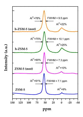
Figure 4. <sup>27</sup>AI MAS NMR spectra of the calcined ZSM-5 samples.
