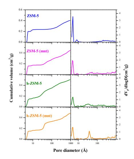
**Figure 2.** Ar adsorption-desorption isotherms at 87.5 K of the ZSM-5 samples: a) cumulative pore volumes and b) pore size distributions, determined by application of the NLDFT model.
