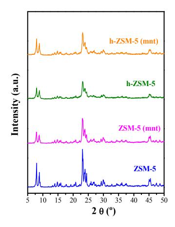
Figure 1. High-angle XRD patterns of the ZSM-5 samples.
