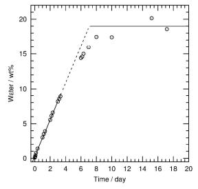
Figure 6: Evolution of the water quantity (expressed in weight percent) in a reline sample in contact with atmosphere (under mixing), as function of time. The average temperature and the atmospheric relative humidity are respectively 21°C and 50%.
