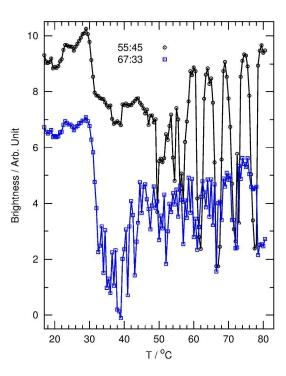
Figure 2: Evolution of the brightness of the 55:45 and 67:33 samples during an experiment in the thermostated bath at a heating rate of 0.25 °C/min. For readability reasons, the brightness of the two samples has been shifted from each other.
