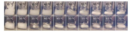
Figure 1: Photographs of 55:45 (top) and 67:33 (bottom) urea: ChCl mixtures taken in the thermostated bath during an experiment at a scanning rate of 0.25 °C/min. After the melting, the stirrer bar is clearly visible in both liquid mixtures.
