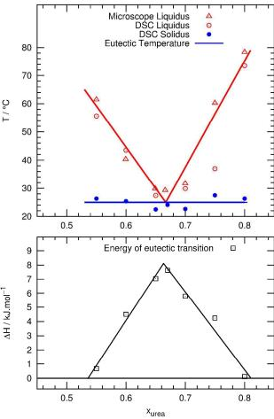
Figure 5: Solid-liquid phase diagram of the system urea: ChCl as function of the urea mole fraction. For clarity reason, only the average temperature is shown when experiments were repeated with two scanning rates. The red lines are only added to help the reader. On the bottom, the Tammann's plot of the enthalpy of the eutectic transition is also given.
