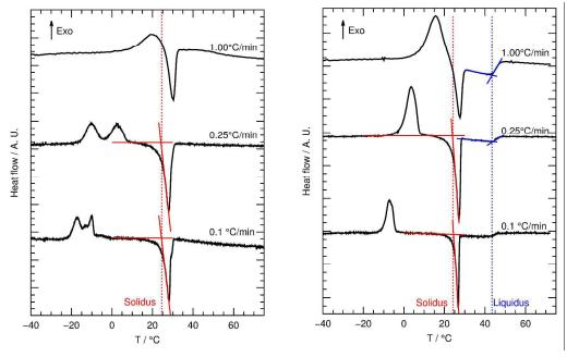
Figure 4: Thermograms of 67:33 (left) and 60:40 (right) samples obtained with scanning rates of 0.1, 0.25 and 1 °C/min. Exothermic peaks (signal up) correspond to crystallization and endothermic ones (signal down) to melting. For readability reasons, the thermograms have been shifted from each other. Construction lines used to obtain the solidus (in red) and liquidus (blue) temperatures are added to the thermograms.
