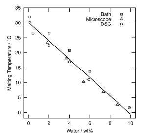
Figure 7: Evolution of the melting point of a 67:33 mixture as a function of the water quantity expressed in wt%. In the thermostated bath, the temperature determined is obtained from the beginning of the decrease of the brightness. With the microscope, it corresponds to the first image without any crystals. With the DSC, the temperature is obtained at the end of the melting determined similarly to the liquidus temperature of the dried samples.
