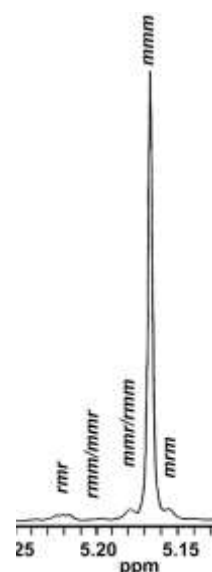
Figure 6. Homonuclear decoupled ^1\text{H NMR} spectrum of the methine part of poly( rac -LA) using 3 at 25 °C, P_m = 0.91 , in \text{CDCl}_3 (Table 2, Entry 6).
