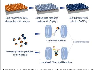
Scheme 1 Schematic illustration of fabrication process of magneto-electric Janus microparticles and their manipulation as well as applications for noble metal reduction reaction.
