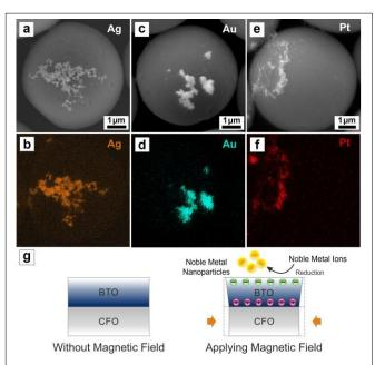
**Figure 2** SEM images (a, c, e) of ME Janus microsphere with noble metal nanoparticles on top after reduction experiments. The corresponding element distribution EDX maps (b, d, f) confirm the composition of the nanoparticles. (g) Schematic illustration of procedures for magneto-electro-chemical reduction of noble metal ions.
